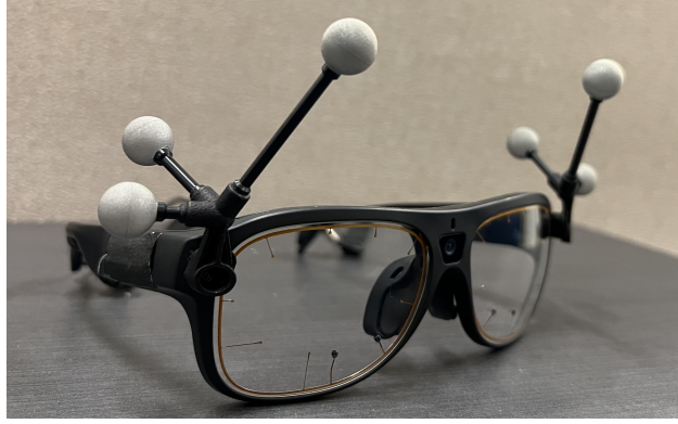
Figure 1.1: Tobii Pro 3 wearable glasses equipped with reflective markers for motion capture integration.
