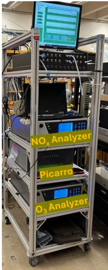
Figure 4.S.2: The Moving rack consists of a multiplexer, NO x , G2509, and O 3 analyzer from top to bottom.
