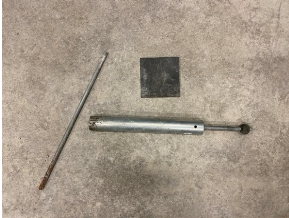
Figure 8: Compaction tools used for casting permeable concrete cylinders and slabs. A large tamping rod, and standard proctor hammer were used for cylinders and a square steel plate with the proctor hammer was used for casting the permeable concrete slabs
