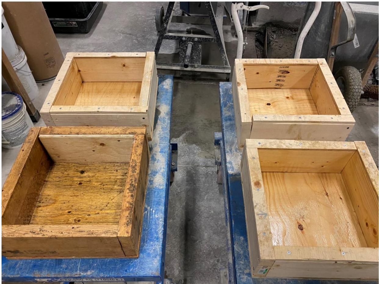
Figure 14: Wooden forms for PCPC slabs.
