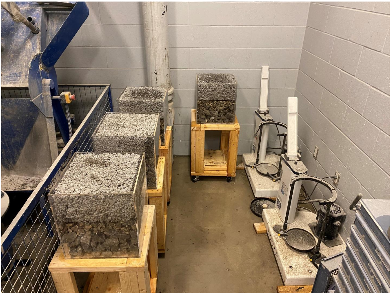
Figure 15: Four lab-scale pavement specimen and their three distinct layers: PCPC slab, base layer, and drainage layer
