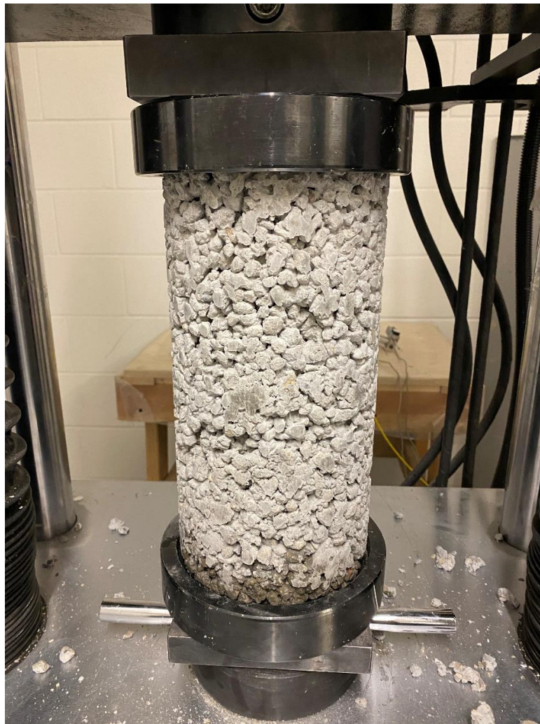
Figure 11: Test setup for measuring compressive strength of a PCPC cylinder with neoprene caps at the ends of the specimen
