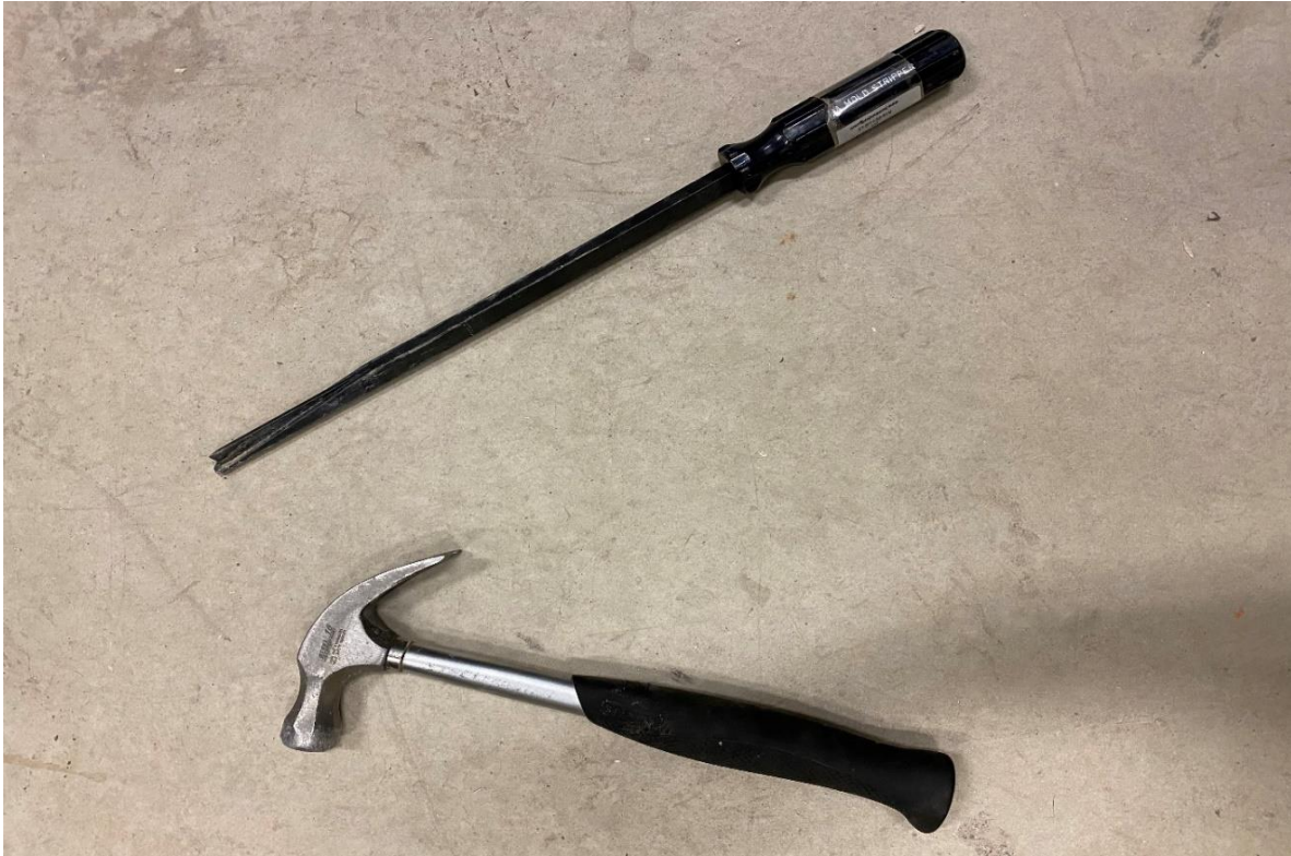
Figure 9: Tools for removing concrete cylinder from their mould. Top: Cylinder mould stripping tool; Bottom: Hammer
