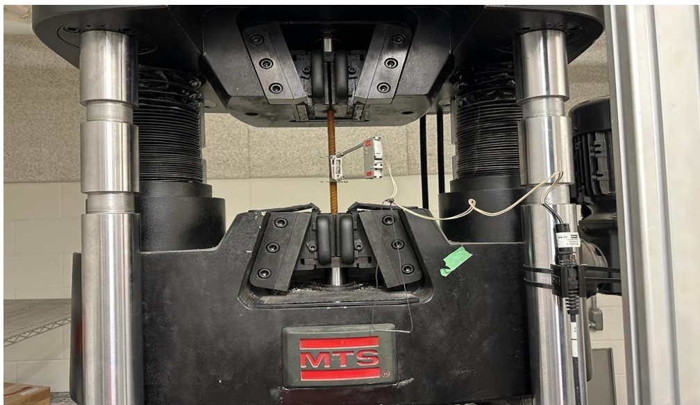
Figure 4.13-Extensometer and Reinforcing Steel Arrangement for the Test
