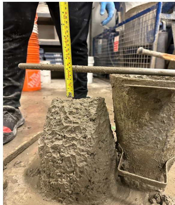
Figure 4.33-Measurement of the Concrete Slump
