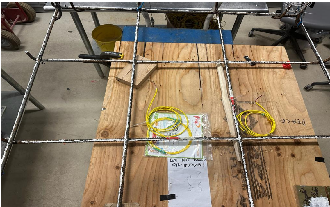
Figure B.18-DFOS After Silicon Glazing
