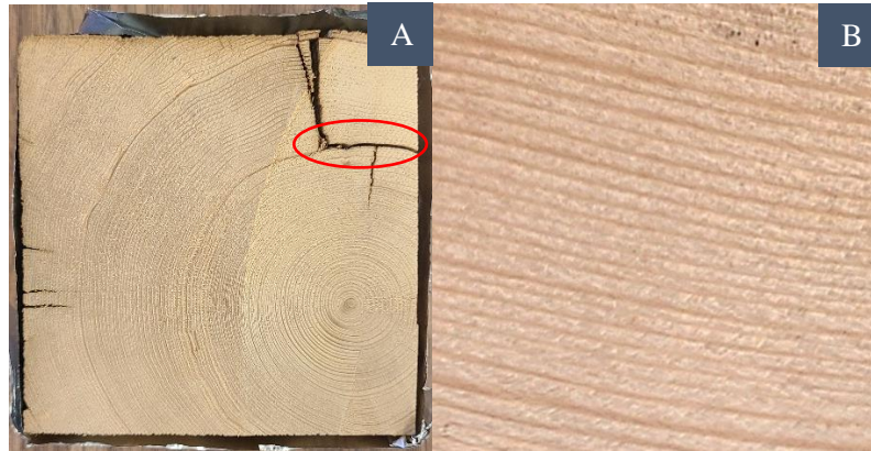
Figure 5-1: Eastern Hemlock. Fig. A shows ring shake. Fig. B cross-grain
