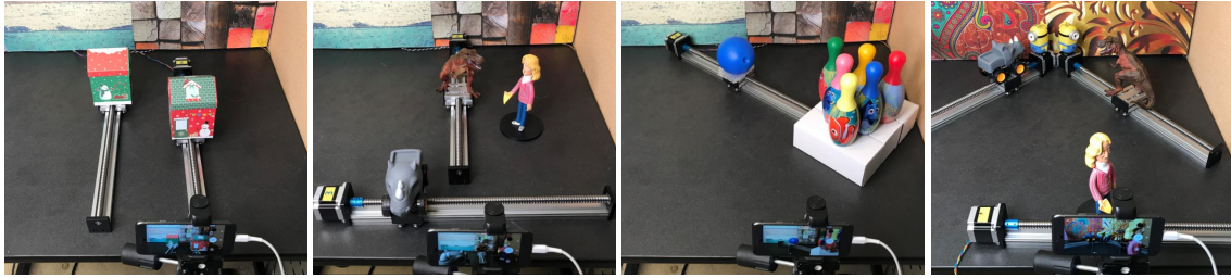
Figure 3.2: A top view of our capture environment. Each shot contains the scene components: linear stage actuators, smartphone camera, tripod, objects, and scene background.
