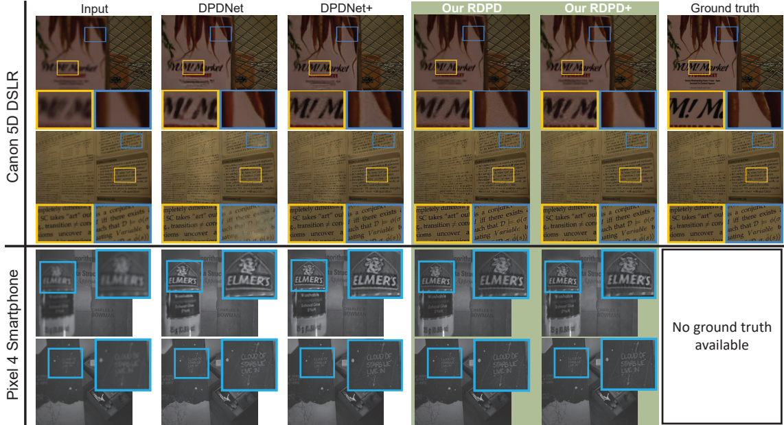
Figure 6.10: Qualitative results. DPDNet [3] is trained on Canon DP data. RDPD is our method trained on synthetically generated DP data only. DPDNet+ and RDPD+ are trained on both Canon and synthetic DP data. In general, RDPD and RDPD+ are able to recover more image details. Interestingly, RDPD trained on synthetic data generalizes well to real data from the two tested cameras. Note that there is no ground truth sharp image for Pixel 4, due to the fact smartphones have fixed aperture and thus a narrow-aperture image cannot be captured to serve as a ground truth image. Additionally, we note that the DP data currently available from the Pixel smartphones are not full-frame, but are limited to only one of the green channels in the raw-Bayer frame.
