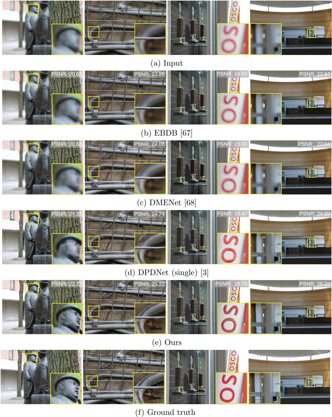
Figure 7.5: Qualitative comparison with single-image defocus deblurring methods on the test set of the Canon DP deblurring dataset [3]. Note that DPDNet was originally introduced to use DP images as input, but the authors in [3] also provided the same model trained on a single image, denoted as DPDNet (single). Our method produces the best quantitative and arguably qualitative results.
