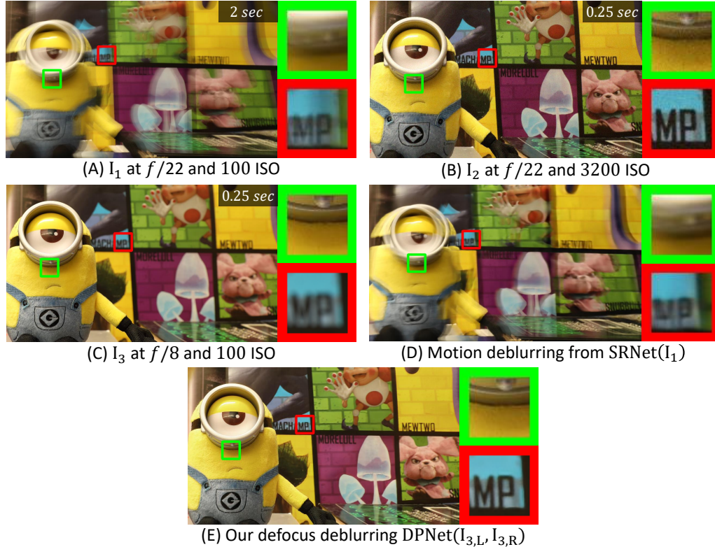
Figure 5.12: Image noise, motion and defocus blur relation with a moving camera. The number shown on each image is the shutter speed. Zoomed-in cropped patches are also provided. (A) shows an image I_1 suffers from motion blur. (B) shows an image I_2 fixes the motion blur by increasing the ISO, however, I_2 has more noise. (C) shows another image I_3 handles the motion blur by increasing the aperture size, nevertheless, I_3 suffers from defocus blur. (D) shows the results of deblurring I_1 using the motion deblurring method SRNet [2]. The image in (E) is the sharp and clean image obtained using our DPNet to deblur I_3 .
