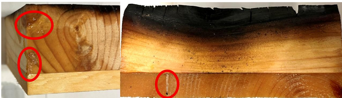
Figure 4.9: Examples of adhesive bleeding occurring during the CLT cone calorimeter tests (circled in red).
