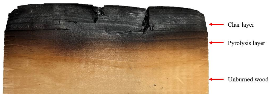
Figure 2.7: Cross section of burned timber showing the char layer.
