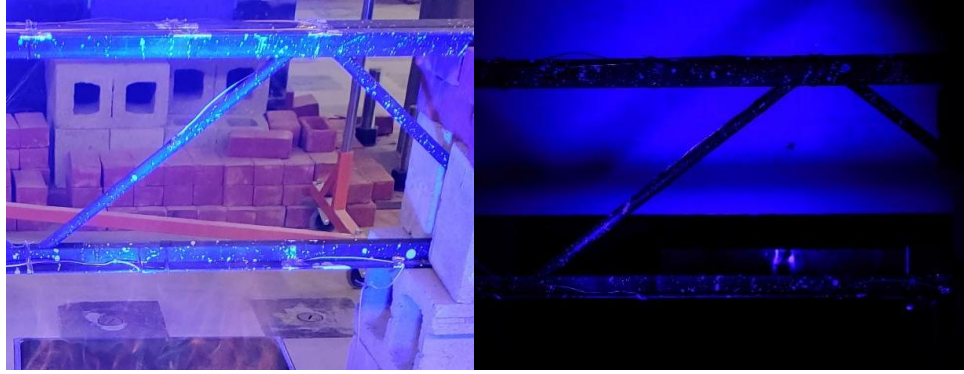
Figure 3.3: Images of a truss exposed to a localized fire before (left) and after (right) using narrow spectrum illumination.
