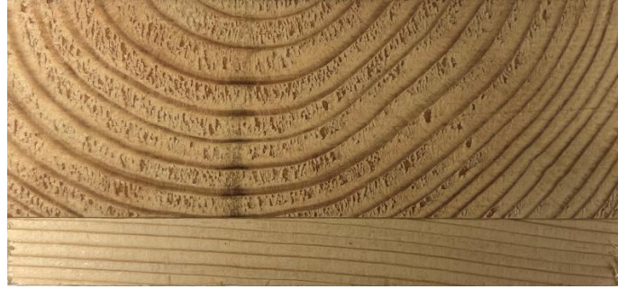
Figure 4.3: Prepared CLT sample prior to cone calorimeter testing.
