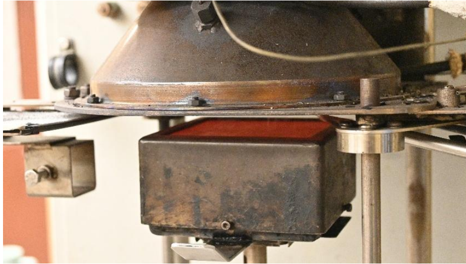
Figure 4.5: Cone calorimeter heating mechanism.
