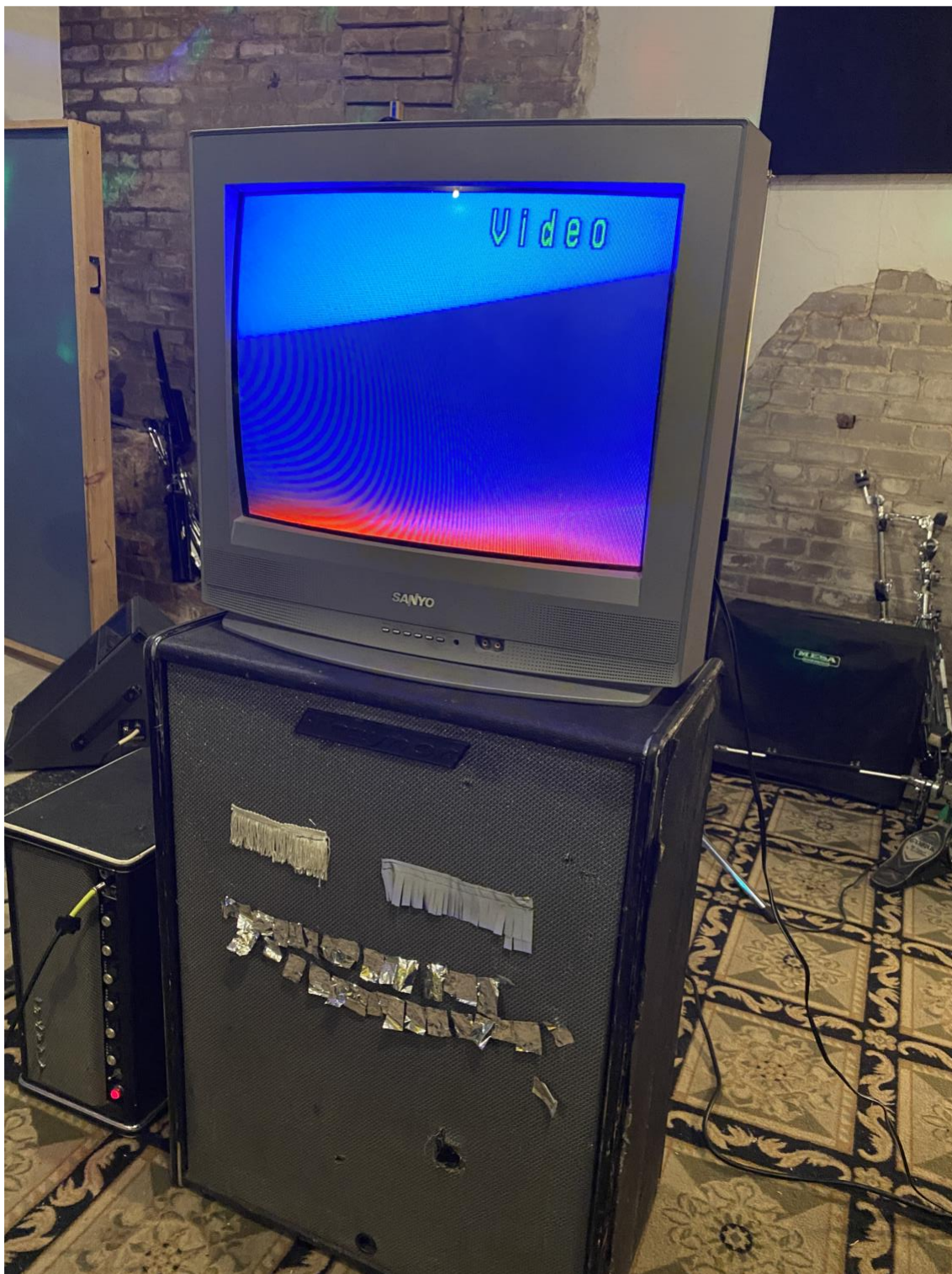
Figure 8. Initial testing of speaker magnet/CRT television interaction.
