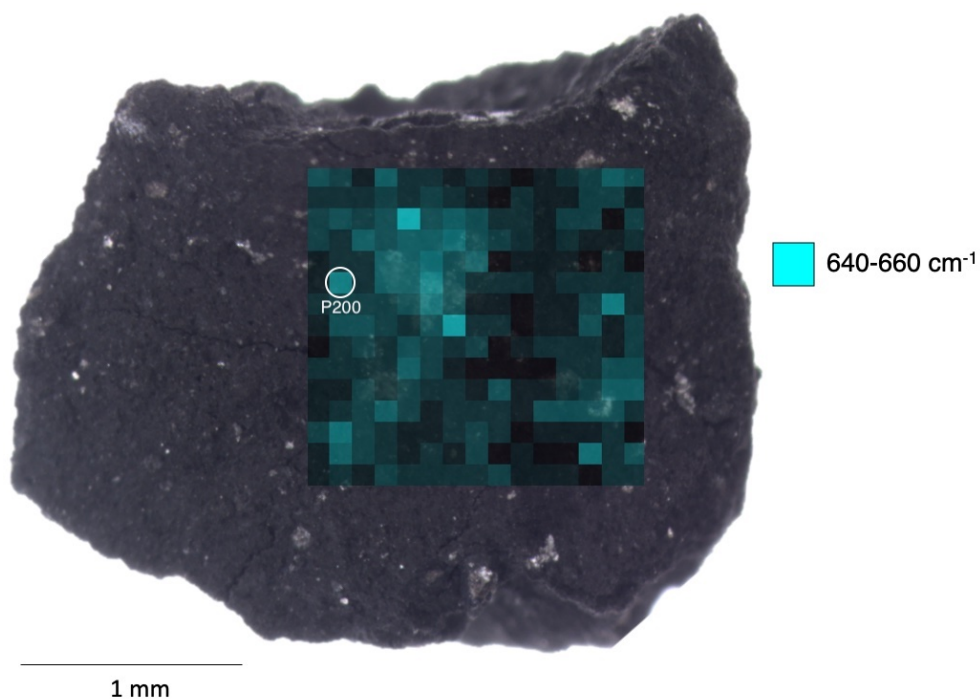
(a) 266 nm Raman map of magnetite-like mineral in Tagish Lake at 650\text{ cm}^{-1} (spectra not baseline corrected).
