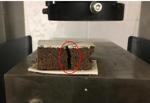
Figure 5-32: Failure crack pattern of GB-20
