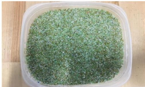
*Figure 3-41: Recycled Crushed Glass (RCG)*
