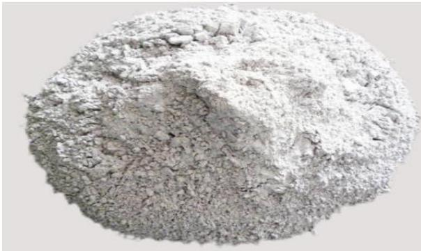
Figure 3-36 :Granulated Blast Furnace Slag (GBFS)
