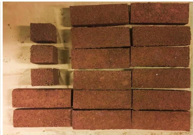
*Figure 4-3: Geo-polymer Bricks (GB-30)*
