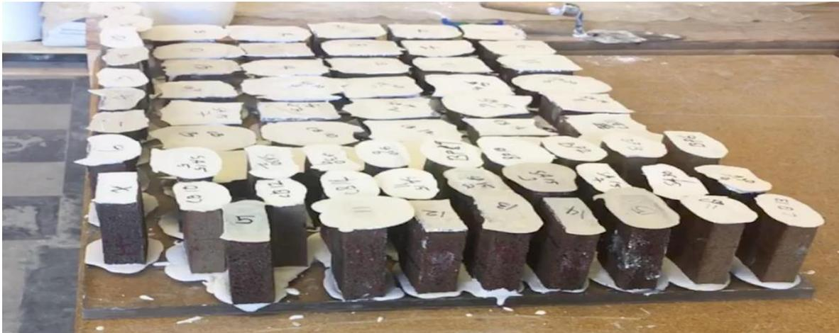
Figure 5-27: The bricks arranged for the drying of gypsum
