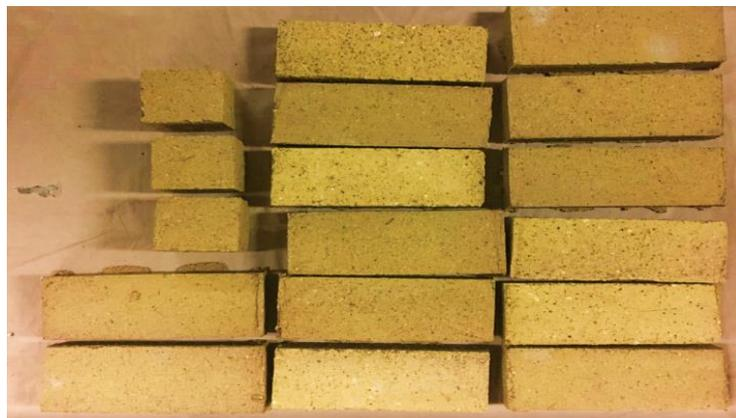
*Figure 4-5: Dried High Bio-Polymer Sludge Bricks (DHBS)*
