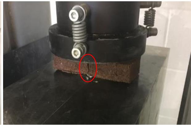
Figure 5-17: Failure crack pattern of GB-20
