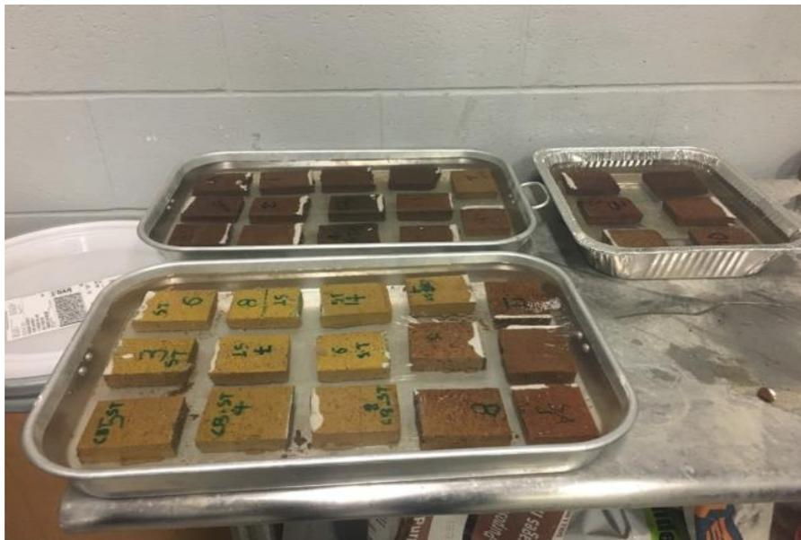
Figure 5-60: Cold-water absorption test
