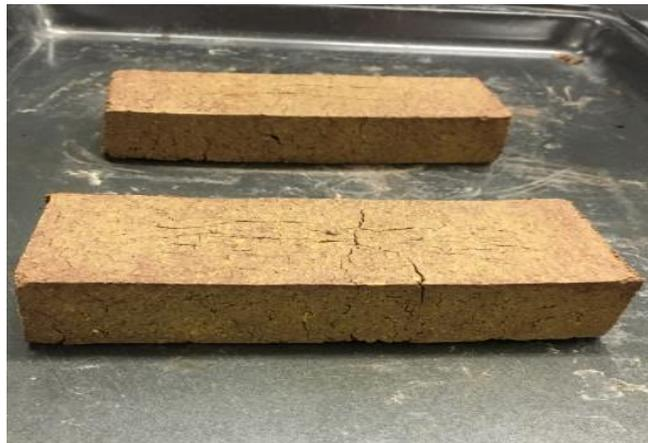
Figure 3-26: Liquid High Biopolymer Sludge Type 2-0.40 Brick (LHBS-2-1)
