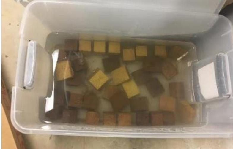
Figure 5-65 : Bricks in the thawing tank
