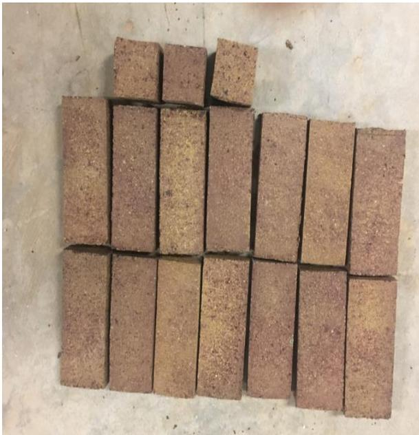
*Figure 4-6 Sewage Sludge Ash Bricks (SSAB-15)*
