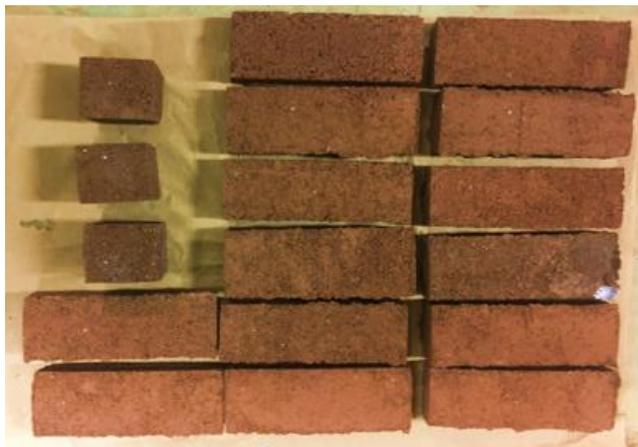
*Figure 4-2: Geo-polymer Bricks (GB-20)*
