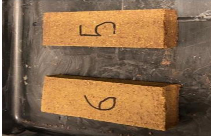
Figure 3-25 :Liquid High Biopolymer Sludge Type 2-0.50 Brick (LHBS-2-0.50)
