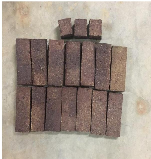
*Figure 4-7 Sewage Sludge Ash Bricks (SSAB-30)*
