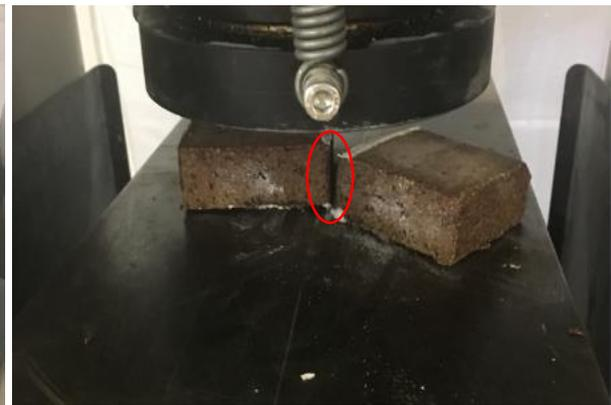
Figure 5-19: Failure crack pattern of GB-40
