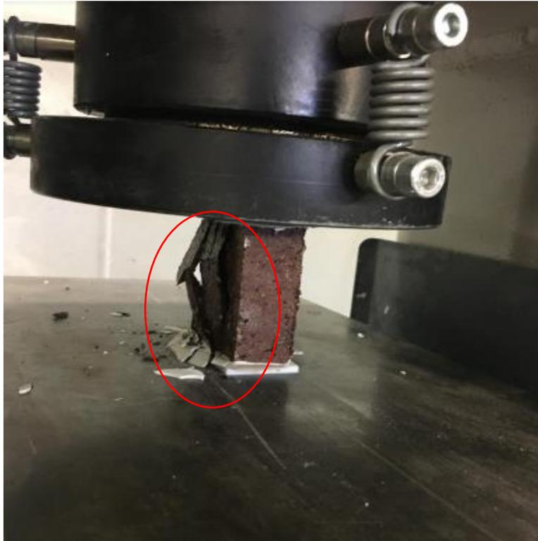
Figure 5-44: Failure crack pattern of SSAB-30
