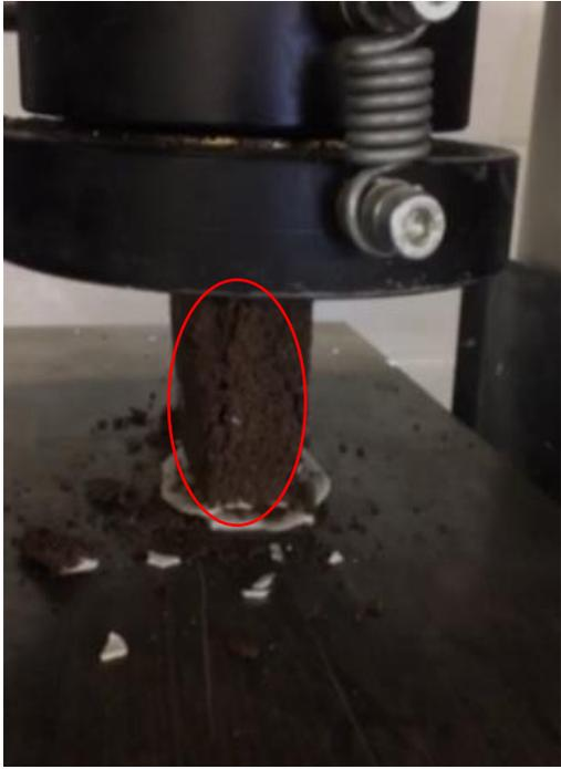
Figure 5-42: Failure crack pattern of GB-40
