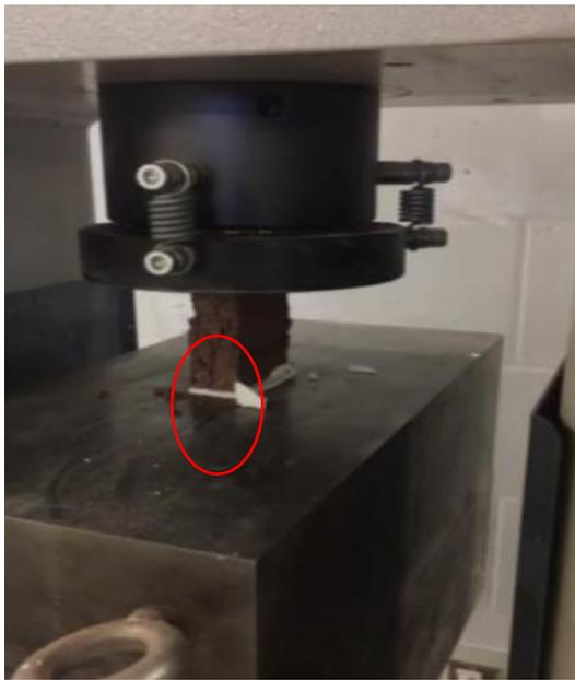
Figure 5-40: Failure crack pattern of GB-20
