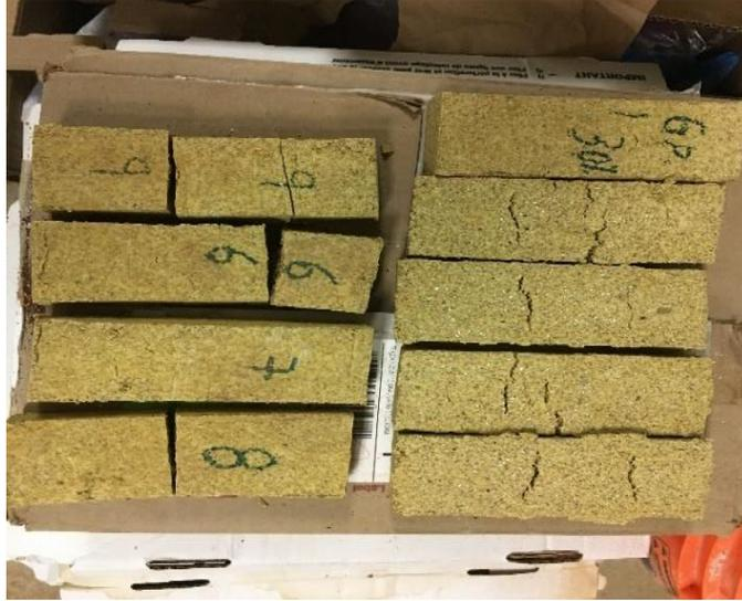
Figure 3-35 :Poraver® Bricks with shale replacement of 30% by weight
