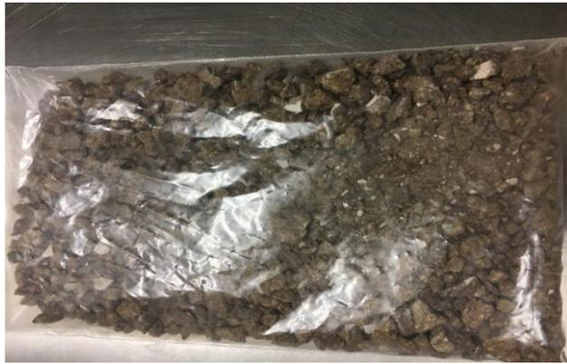
*Figure 3-51: Crushed Bricks*
