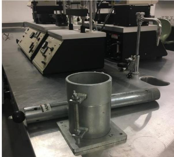
Figure 3-10 :Standard proctor compaction test apparatus
