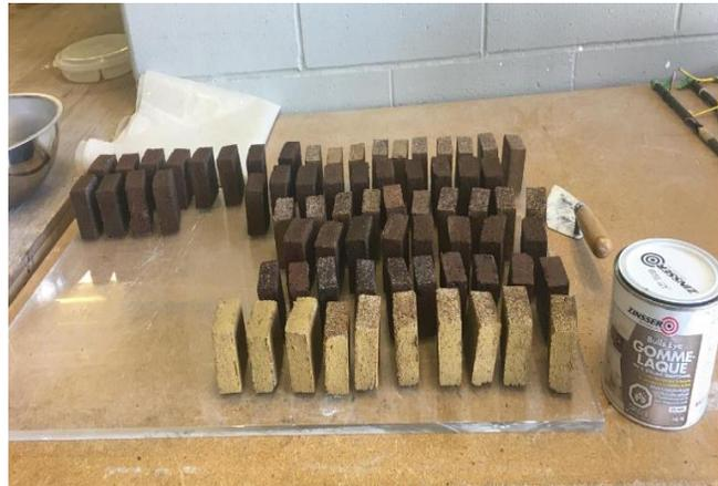
Figure 5-25: Sealant used for Gypsum capping (Zinsser.com) Figure 5-26 : Shellacked bricks before the gypsum capping
