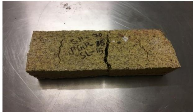
Figure 3-37 :Shale-Poraver®-Slag Bricks (SPSB)
