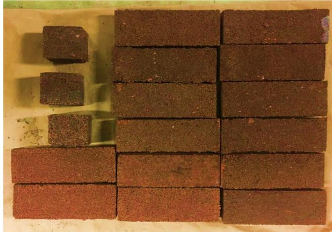
*Figure 4-4: Geo-polymer Bricks (GB-40)*
