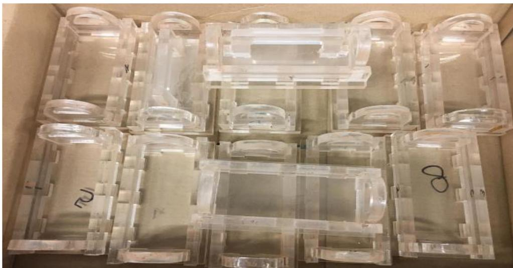
*Figure 4-1: Fourteen Acrylic brick molds made for the main phase of the experimental research*
