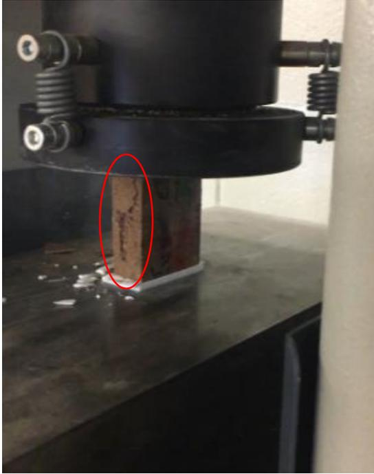
Figure 5-38: Failure crack pattern of Control bricks (CB)
