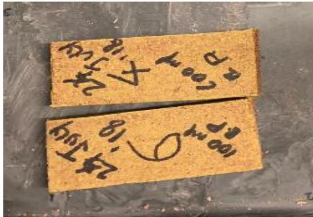
Figure 3-21 :Liquid High Biopolymer Sludge Type 1-0.4 Brick(LHBS-1-0.4)
