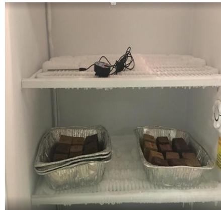
Figure 5-67: Bricks inside the freezing chamber
