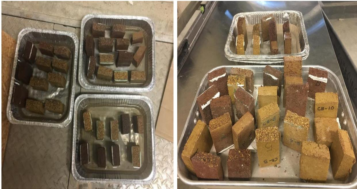
Figure 5-64 (a): The bricks placed in the tray for efflorescence test (b): Appearance of the bricks after the efflorescence test.
