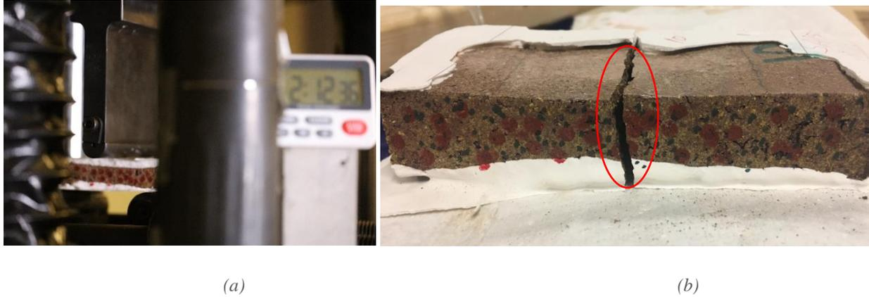
Figure-5-11 (a) Test Set up (b) :Failure Pattern of sewage sludge ash Brick (SSAB-30)
