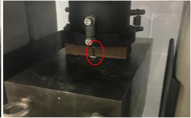
Figure 5-15 : Failure crack pattern of Control bricks (CB) Figure 5-16 : Failure crack pattern of DHBS
