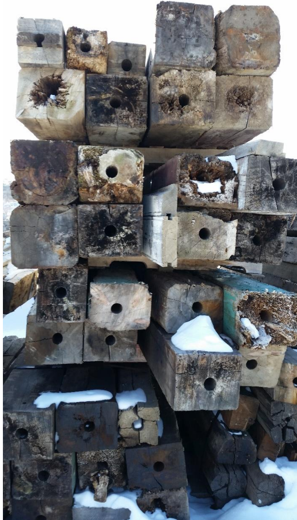
Figure 4.3. Improper storage of heritage timber materials.
