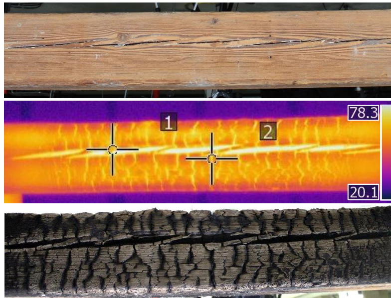
Figure 4.8. Side A crack progression before (top) and after fire (middle and bottom) on Heritage 2 (identifiable markings were recorded temperature markers and scale is in °C).
