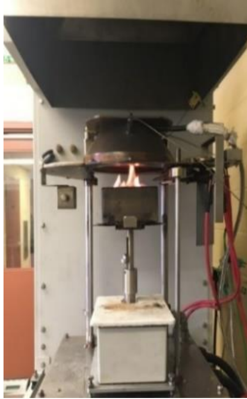
Figure 4.7. Cone calorimeter test setup.
