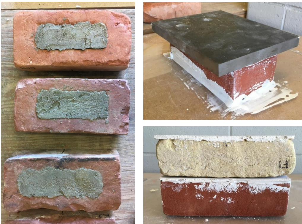
Figure 5.5. Mortar filling and plaster capping of clay brick samples.
