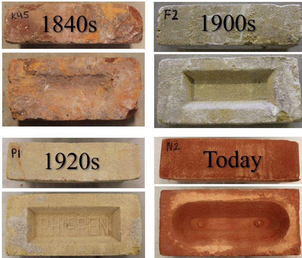
Figure 5.2. Brick samples from the 4 eras of Canadian brick masonry construction.
