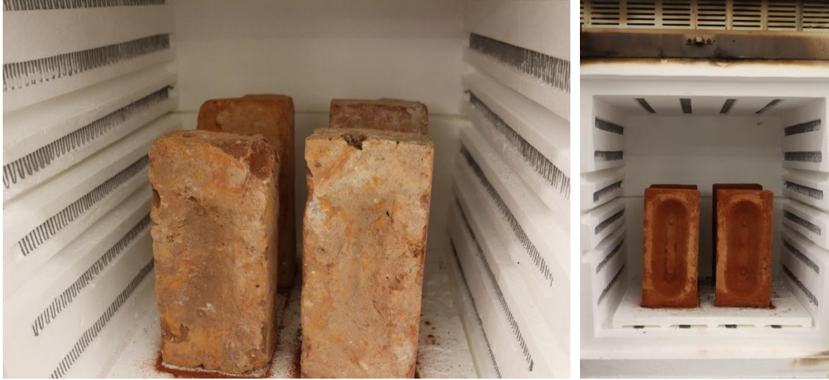
Figure 5.3. Brick configuration in the furnace (1840s and new (2010s) bricks).
