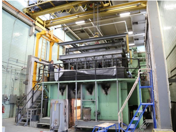
Figure 2.3. A standard fire furnace of fixed dimensions (photo by John Gales used with permission).
