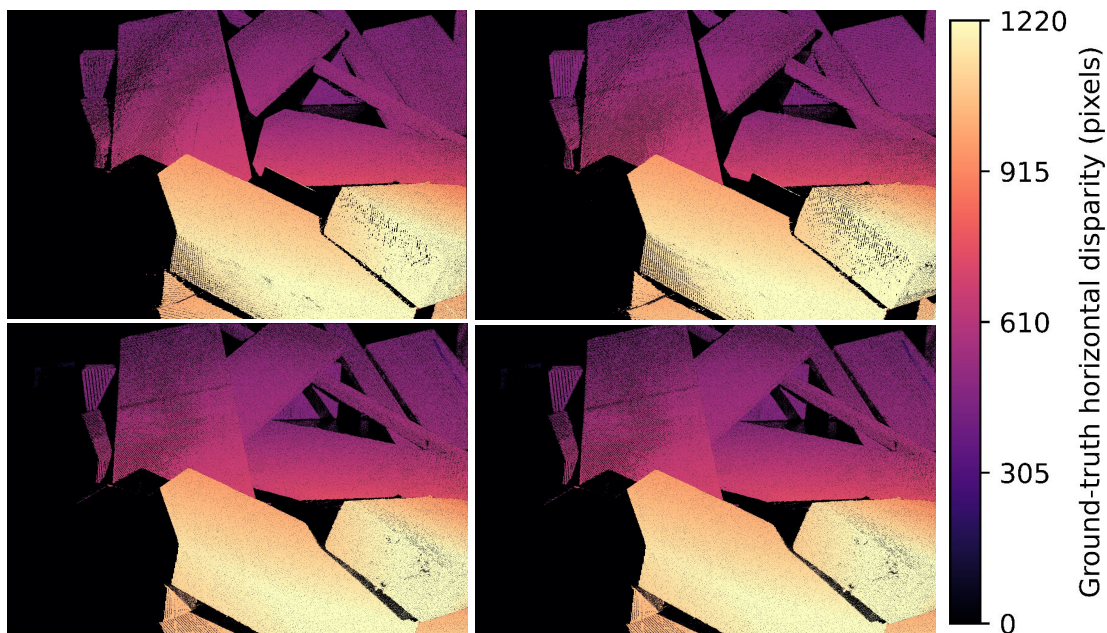
Figure 4.8: Example disparity outputs after decoding. Each output is the result of one set of 46 Gray-code images.
