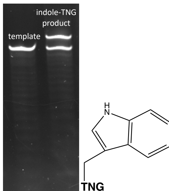
Figure 20: 10% denaturing PAGE gel (150V, 55 °C, 40 min) of the LOOPER product after 13 incorporations of indole-TNG trimers ligated to generate the full-length product. The image on the right is the general structure of indole-TNG.
