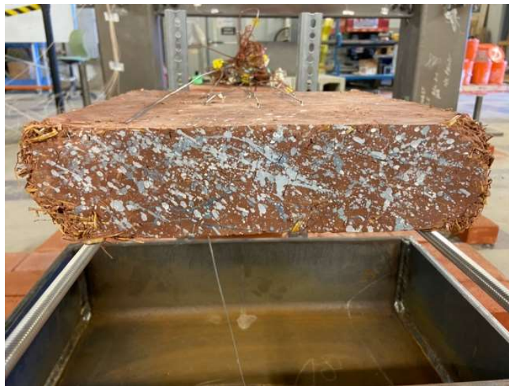
Figure 6.2. Example of painting pattern for Digital Image Correlation
