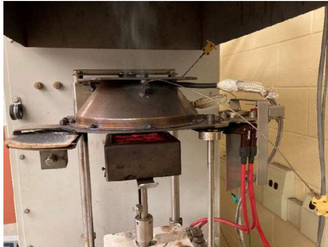
Figure 2.2. Cone Calorimeter test performed in the University of Waterloo. (Photo by Hannah Carton, with permission)
