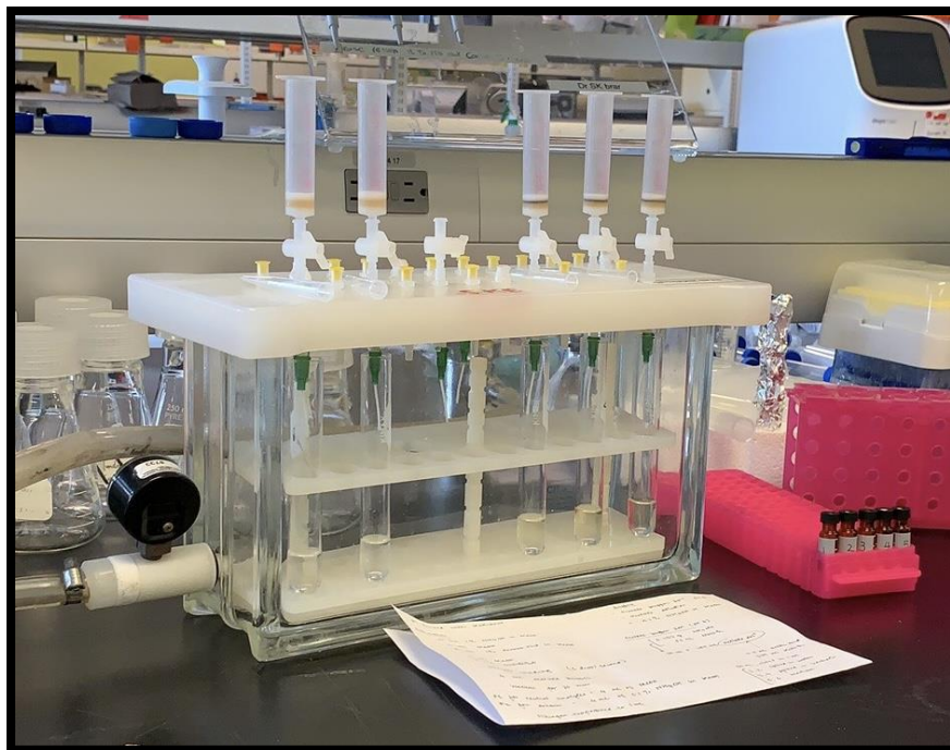
Figure 7: Solid phase extraction of PFCA compound in landfill leachate
