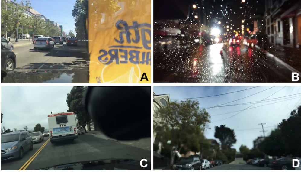
Figure 4.2: Examples of BDD-A videos with image quality issues: A) reflection on the windshield, B) image out of focus, C) camera tilted and partially obstructed, D) camera tilted up, blurry artifacts.
