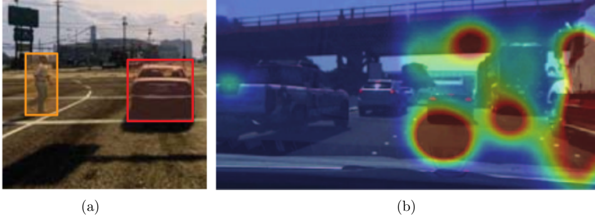
Figure 3.6: Visualized spatial attention weights: a) object-level, b) pixel-wise. Sources: a) [446], b) [444].
