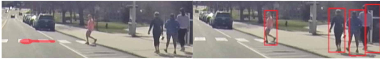
Figure 2.14: Augmented reality visualizations used to guide the driver’s gaze. Left: “virtual shadow” is a less intrusive visualization that leads attention to the pedestrian about to cross. Right: bounding boxes drawn around every pedestrian create visual noise, so the pedestrian about to cross is not immediately apparent. Source: [307].
