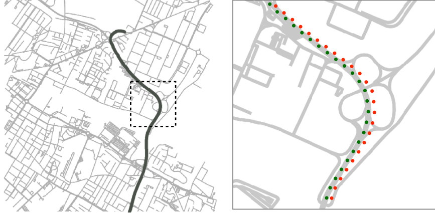
Figure 6.3: Example of the map and route inferred from DR(eye)VE GPS data. Left: street network with overlaid route traveled by the vehicle. Right: enlarged portion of the map shows map matching the original noisy GPS coordinates (shown in red) to the street network (green). Map colors are inverted here for readability. For use in training and inference, street network and route are rendered as white lines on a black background.
