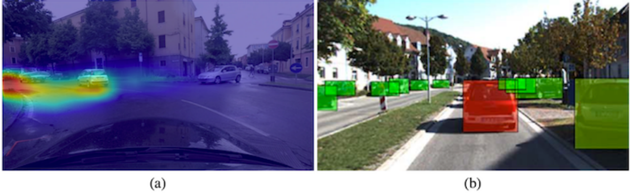
Figure 3.5: Sample outputs of driver gaze estimation algorithms. a) Pixel-level saliency map for vehicle performing a left turn. b) Visualization of object-level importance scores for vehicle following. Red color indicates higher relevance/importance in both images. Sources: a) [422], b) [425].
