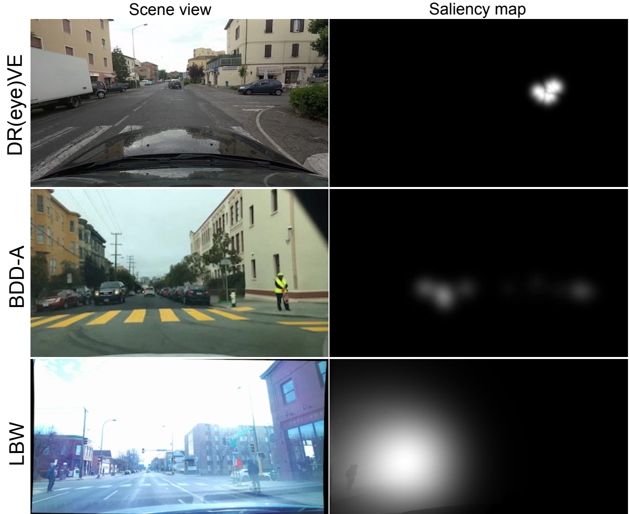
Figure 4.12: Scene images from each dataset and corresponding ground truth saliency maps. Note that in DR(eye)VE and BDD-A, saliency maps are more representative of foveal vision and combine multiple fixations. In LBW, a single fixation is used to generate a saliency map which covers part of the peripheral visual field.
