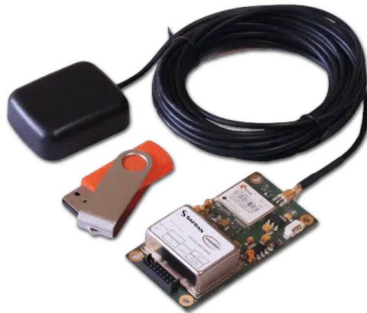
Figure 5.1: GXClock-500 package containing a u-Blox low-cost GNSS receiver chip and patch antenna
