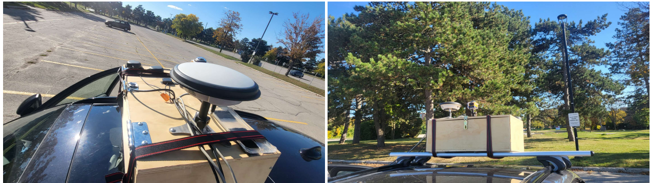
Figure 4.3: Roving sensors integrated with the vehicle rooftop
