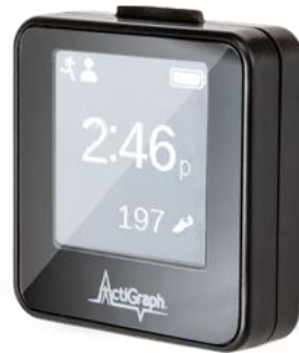
Figure 4.3 The ActiGraph GT9X Link (ActiGraph™, Pensacola, FL, USA) was the activity monitoring device that participants were directed to wear on their right hip for seven consecutive days during waking hours.
