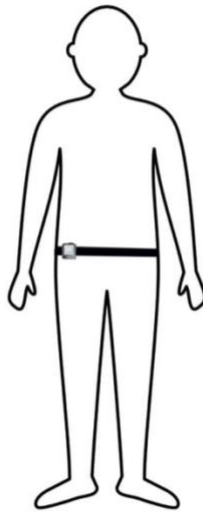
Figure 4.4 The ActiGraph GT9X Link activity monitors were strapped onto the participant's right hip with an adjustable elastic belt and participants were instructed to wear the activity monitor as such during waking hours for the duration of the seven-day collection period.
