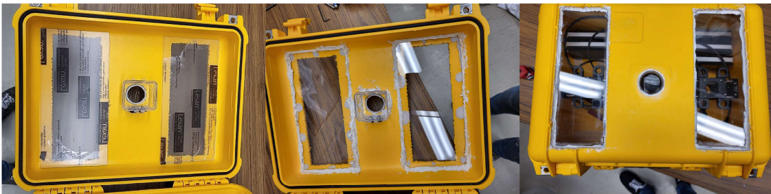
Figure 4.12: Left: Polycarbonate windows were sized to the correct size of the two rectangular laser window location. The window for the camera was a panoramic camera case. The hole for this window was filed down to ensure a snug fit with the window.
