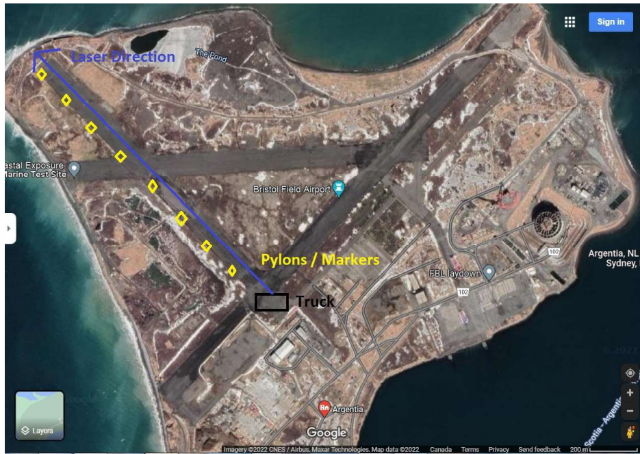
Figure 4.15: A map of the Argentia runway courtesy of WOOD PLC. This was used to convey to port authority where the lasers would be located with respect to port traffic. The black rectangle represents our starting point with the WOOD PLC truck and pylons would be used to mark down the runway. To avoid construction on the NE side of the port, the lasers could not point that way, but in the direction of the blue line.
