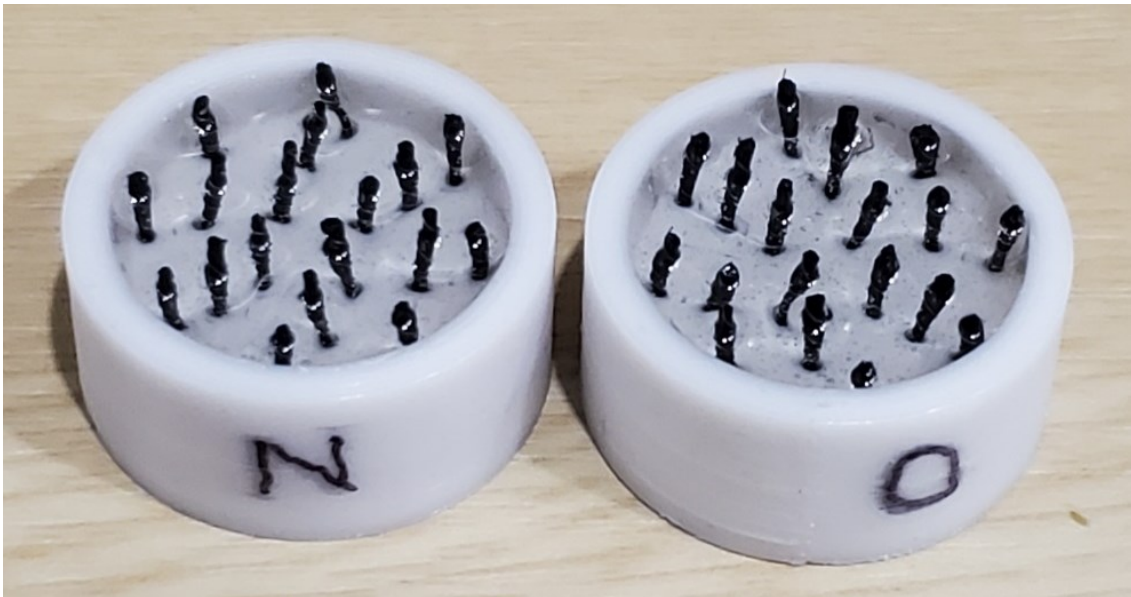
Figure 3-3: K13D2U tow embedded in epoxy resin
