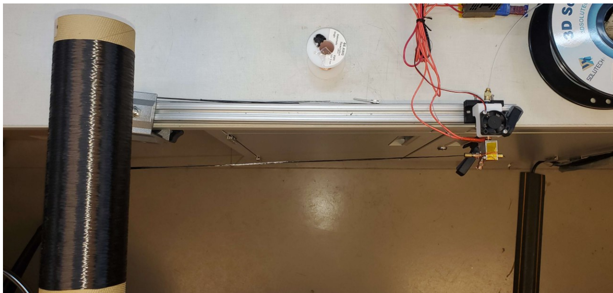
Figure 5-3: Top-down view of fiber coating apparatus
