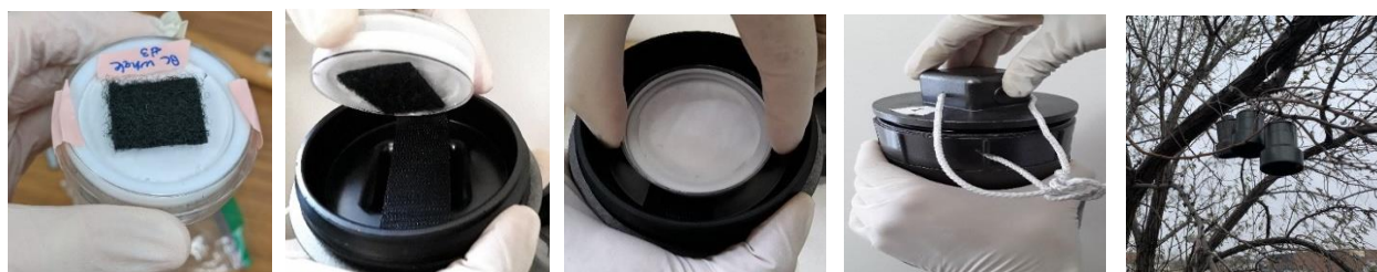
Figure S2.1 From left to right: steps for the deployment of PAS. From right to left: steps for the collection of PAS (Carmichael, 2022).
