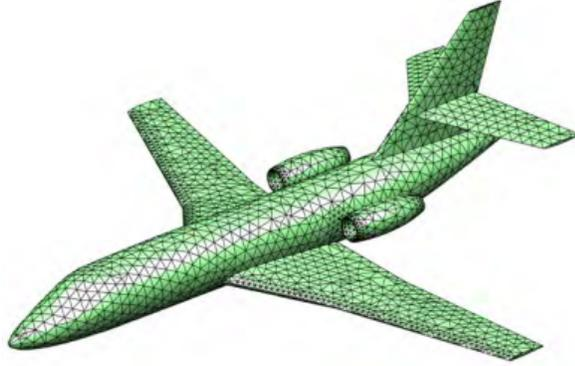
Fig. 1.3 The discretization, or mesh, of a generic aircraft (Image source: [7])
