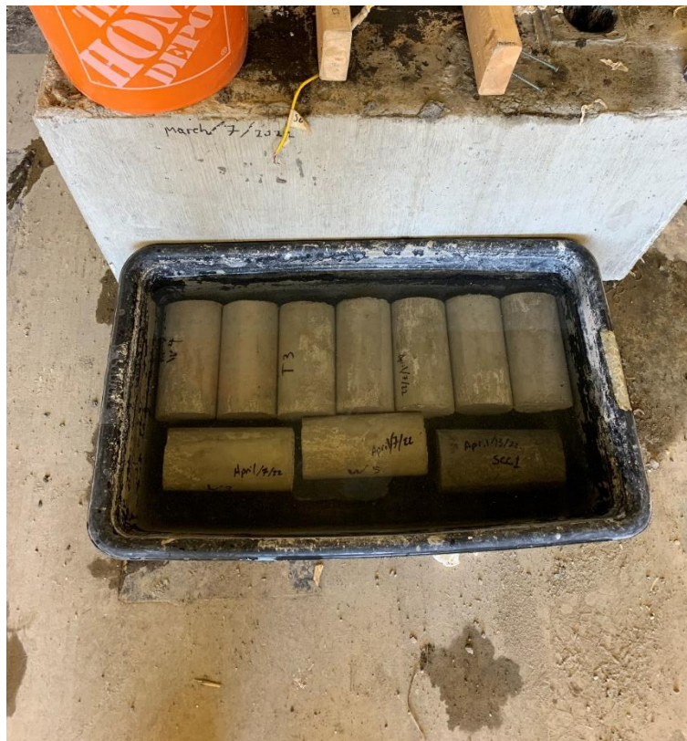
Figure 8.15: Cylinders Placed in Water Bath After Demolding
