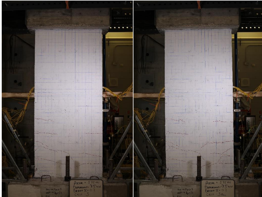
Figure 4.7: Wall at 0.3% Drift (Push on the Left, Pull on the Right)
