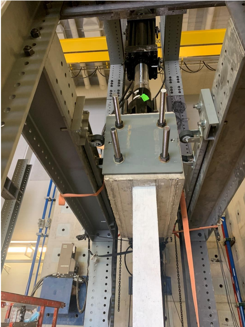
Figure 8.52: Securing Steel Plate and Threaded Rods to Cap Beam
