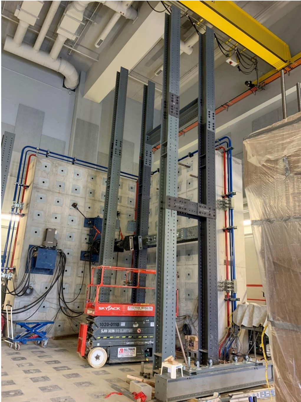
Figure 8.45: Adding Column Extensions to Columns and Upper Cross Beam
