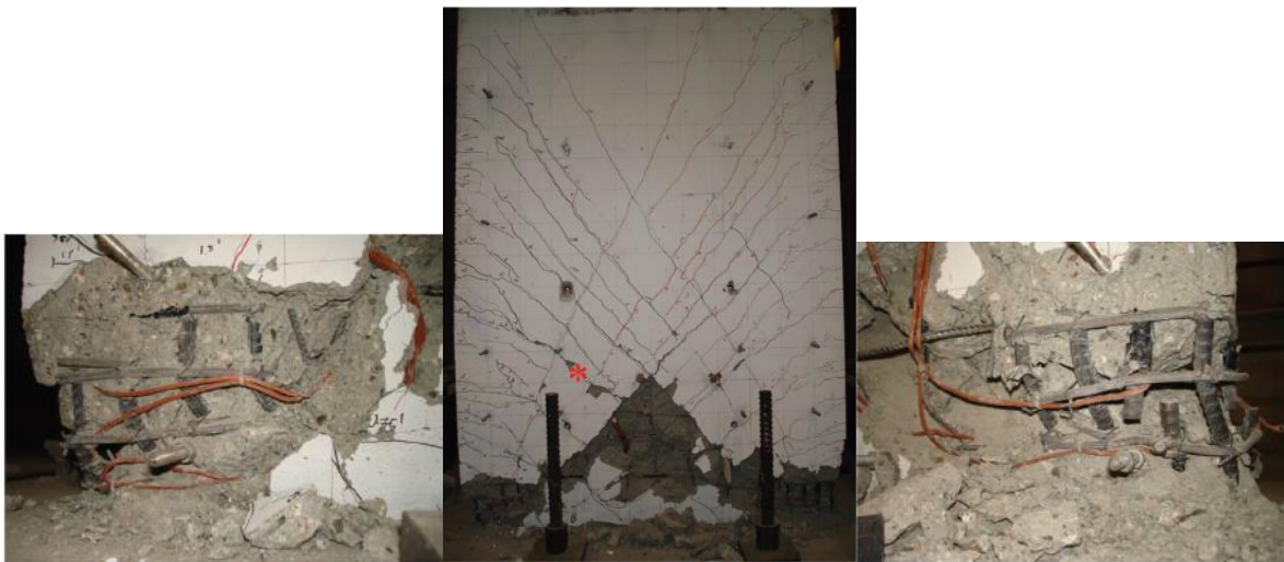
Figure 2.4: Failure of Wall RW-A20-P10-S38 and boundary regions [19]
