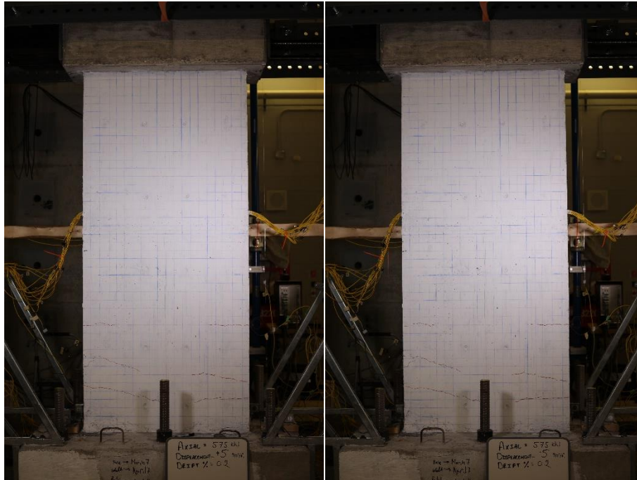
Figure 4.6: Wall at 0.2% Drift (Push on the Left, Pull on the Right)
