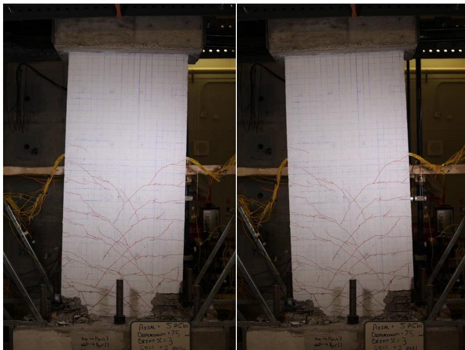
Figure 4.14: Wall at 3.0% Drift (Push on the Left, Pull on the Right)
