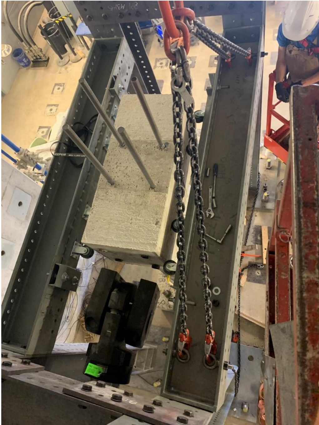
Figure 8.47: Securing Front Cross Beam with Rollers
