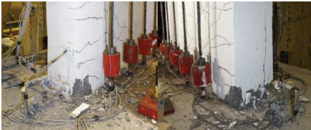
Figure 2.13: Boundary Regions of Figure 2.12 after completion of testing [28]
