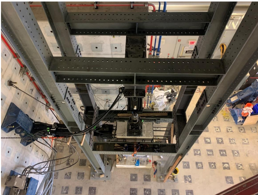
Figure 8.50: Test Frame with Gravity Actuator, Prior to Adding Short Direction Beams, Top View
