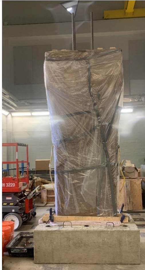
Figure 3.10: Wetting Process for Wall and Cylinders (bottom left in black bin)
