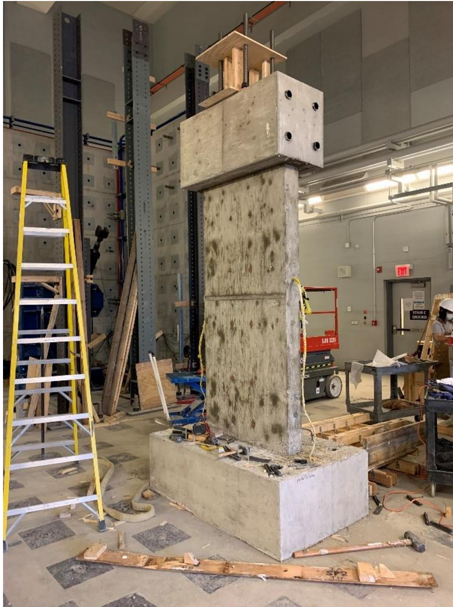
Figure 8.22: Front of Wall After Removal of Formwork
