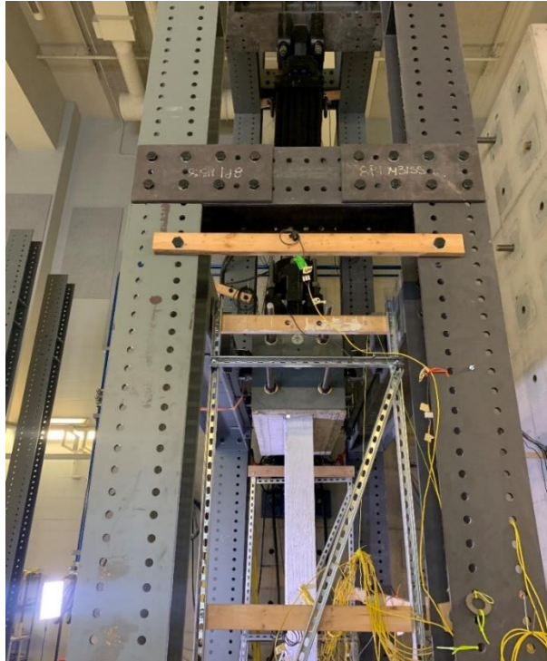
Figure 6.23: Out-of-Plane Lean of the Wall and Actuator during Testing
