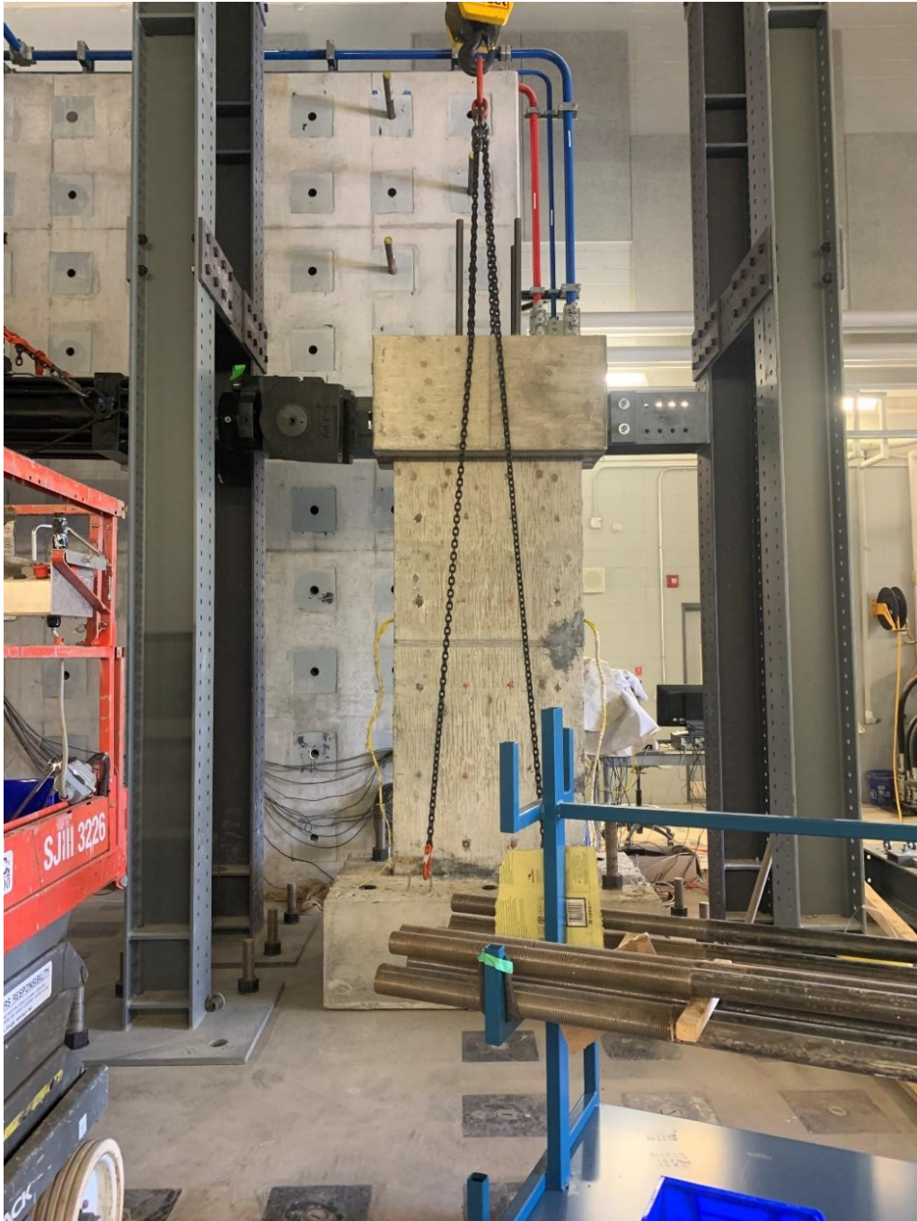
Figure 8.46: Moving Wall into Place
