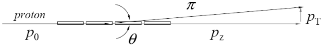
Figure 2.9: Proton impinging on segmented target and producing a pion [68].
