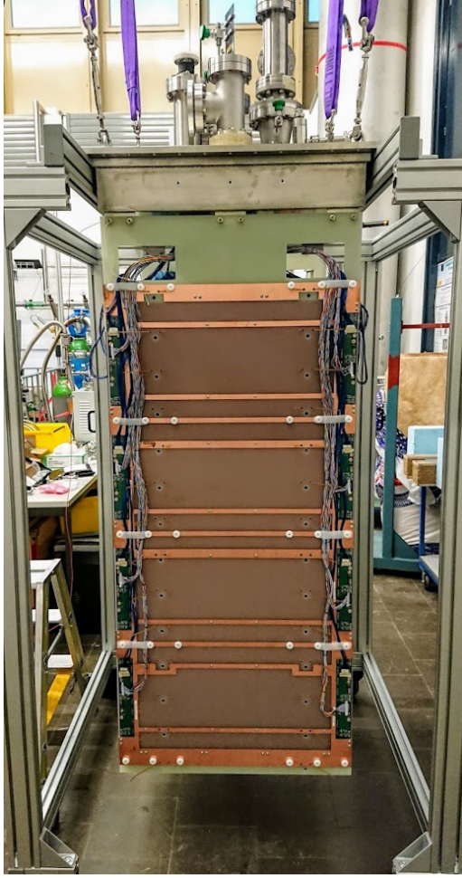
Figure 5.4: Module-0 without its G10 sleeve (left), above the liquid argon cryostat (right).
