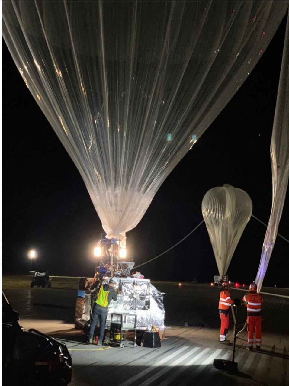
Figure 2.7. Pictured in the foreground is a smaller balloon used to keep the attached gondola steady upon launch. In the background is the larger balloon being inflated to launch. The larger balloon expanded even further as it ascended into the stratosphere.
