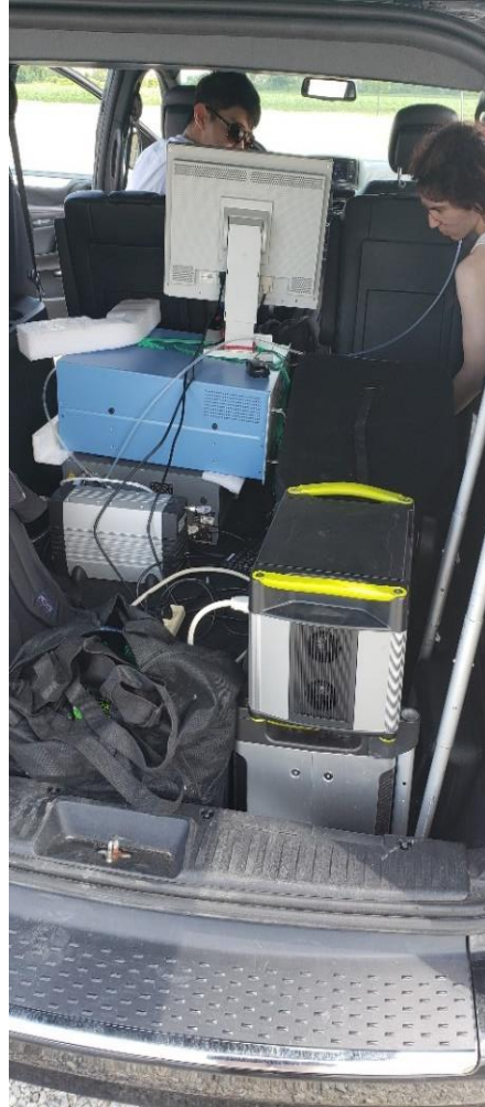
Figure 12. Setup of the Picarro CDRS and Thermo Fisher 43i in the van used for the Sarnia field study.
