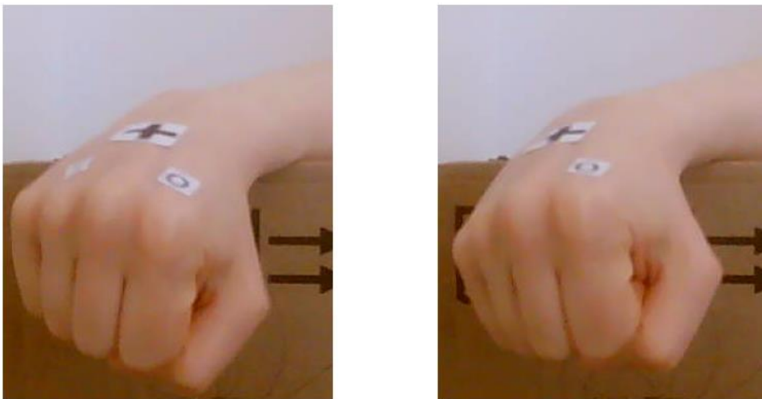
Figure 4.16 Another real environment example is from the side camera's point of view. Here, the system estimated roll at -25.87 degrees (counterclockwise)
