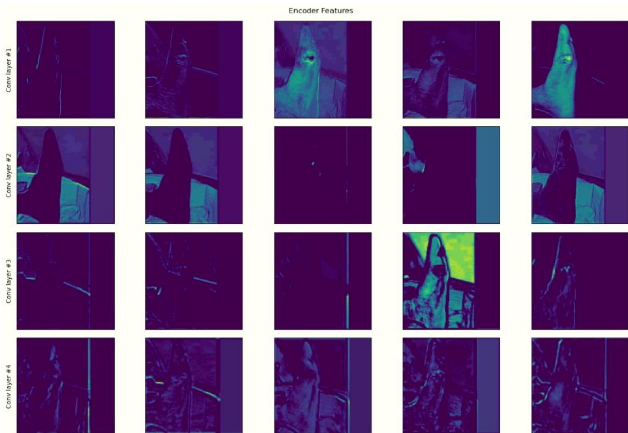
Figure 3.17 Encoder features from the first to the fourth convolution layer (rows 1-4, accordingly). We can spot how features change from low-level to high-level details: background/foreground extraction (rows 1-2), edges detection (row 4)
