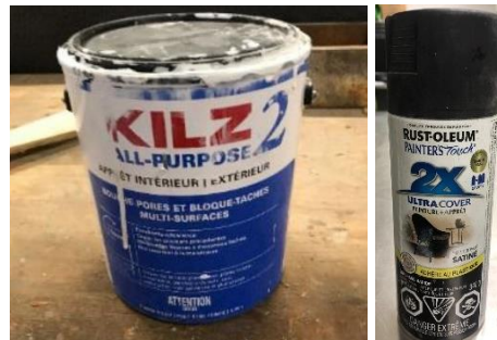
Figure 5.27. White Kilz primer used for coating the specimen's surfaces and Rust-Oleum black spray used for speckles.
