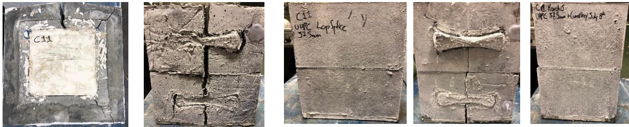
Figure 5.40. Specimen C11, precast jacket with curved key, after testing.
