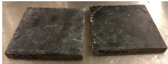
Figure 5.31. Steel loading plates used on top and bottom of the Retrofitted Columns.
