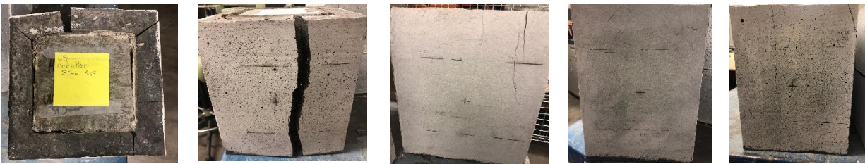
Figure 5.39. Specimen C8, cast-in place jacket, after testing.
