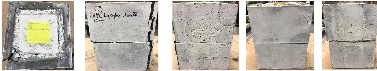
Figure 5.48. Specimen C3, precast jacket with Lap Splice connection, after testing.
