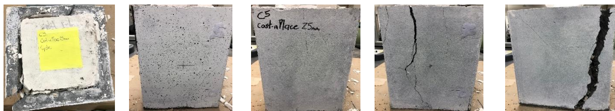
Figure 5.47. Specimen C5, cast-in place jacket, after testing.
