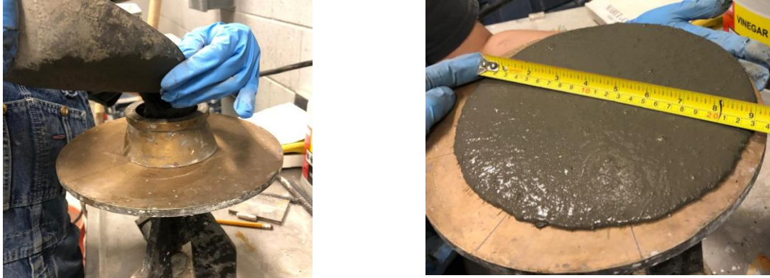
Figure 4.2. UHPFRC CEK2 flow test.
