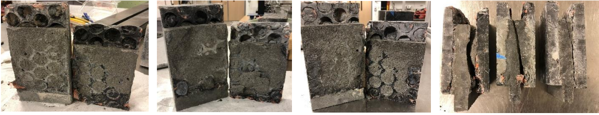
Figure 5.56. Sandwich Specimens after testing under axil load at the top surface of the non-shrink grout.
