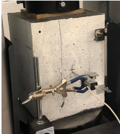
Figure 5.38. Rotation of specimen C8 due to dimensions and space limitations. Only DTs were place on the front and back face of the Retrofitted Column, the LVDTs remain in position.
