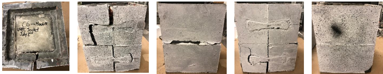
Figure 5.35. Specimen C6, precast UHPFRC Jacket with Curved Key, after testing.
