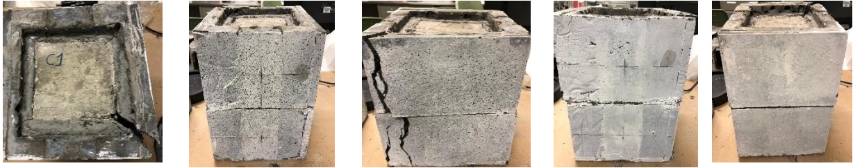
Figure 5.41. Specimen C1, precast jacket with lap splice connection, after testing.
