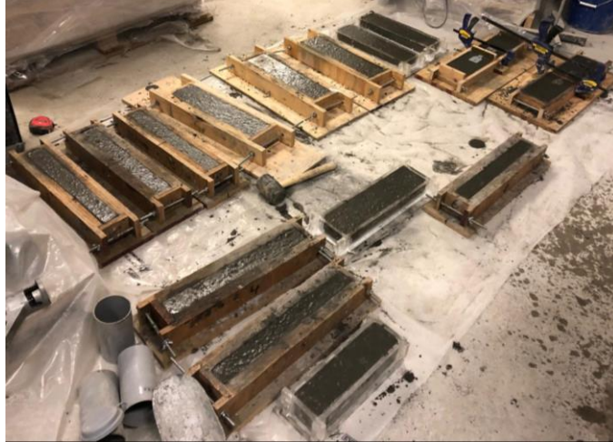
Figure 4.3. CEK2 specimens immediately after casting.
