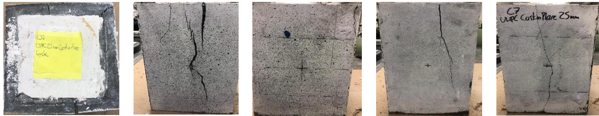
Figure 5.46. Specimen C7, cast-in place jacket, after testing.
