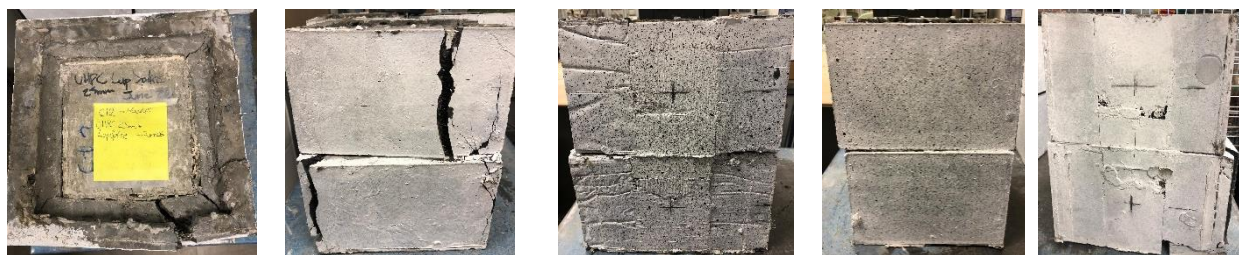
Figure 5.37. Specimen C12, precast jacket with Lap Splice Connection, after testing.
