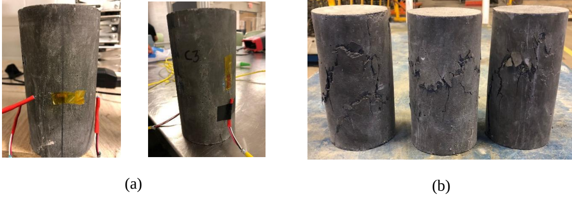
Figure 4.6. (a) Cylindrical specimens setup with strain gauges to obtain values of compressive strength, Poisson's Ratio and Modulus of Elasticity, (b) mode of failure of the cylindrical specimens after testing in the displacement controlled machine.
