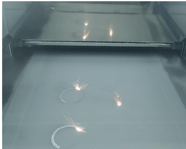
Figure 2.15. Example of a printing process inside a RENISHAW AM 500.
