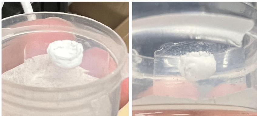
**Figure 4.1:** Cylindrical Silica aerogel sample (1.5 cm in diameter) displaying internal structural collapse from a droplet of water placed atop its surface.
