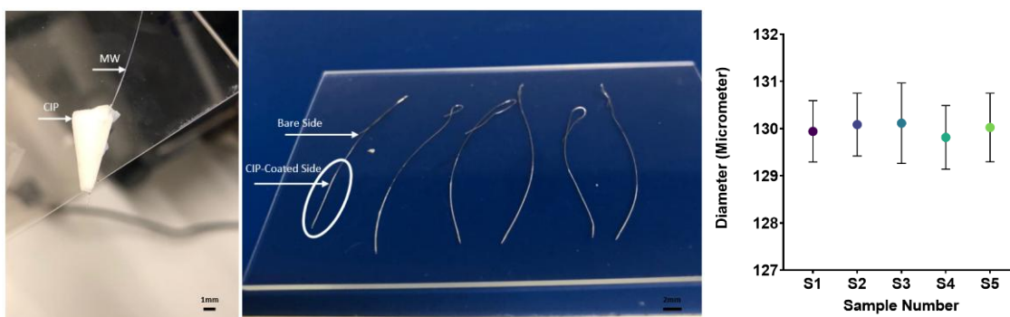
Fig. A1. Left) Polymerized CIP with a MW immobilized inside it after removal from the containing tube. Middle) Different CIP-MWs after removal from the polymer bulk. The coated and bare sides of MWs are labeled. Right) Diameter of five replicated 4-CIP-MW samples showing reproducible CIP coatings[149].
