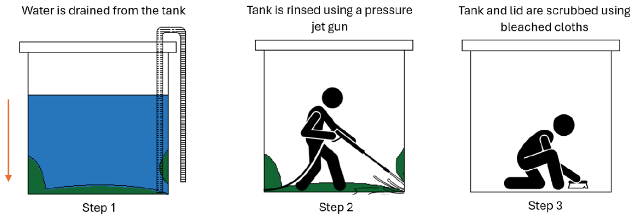
Figure 3-5: Cleaning process of cisterns
