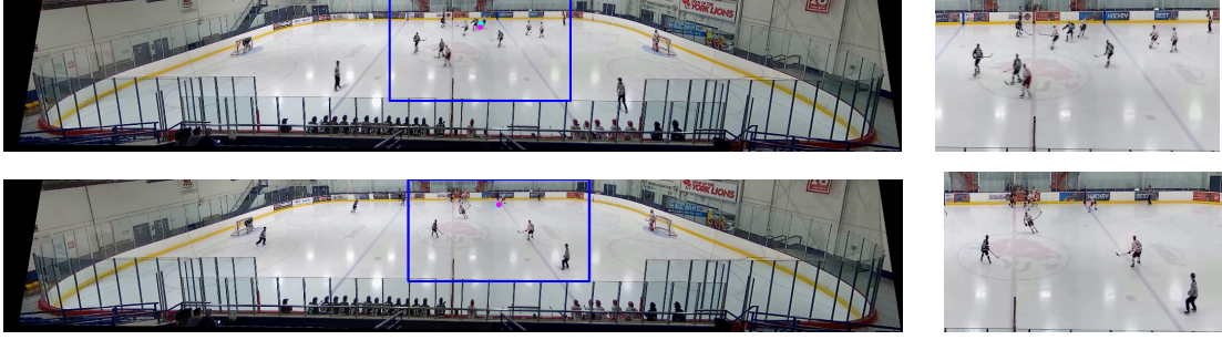
Figure 2.16: Left: Sample results for test images from Camera 2. Cyan and pink dots indicate ground truth puck location and the puck location estimated by APT2 + smoothing, respectively. The blue rectangle indicates the 1280 \times 720 crop region. Right: Corresponding zoomed-in view.
