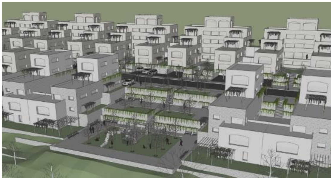
Figure 4 Rendering of a typical urban block in Tantour per Plan 44: pedestrian path system connects different blocks and crosses inner courtyards. Source: Eran Mebel Architects with permission.
