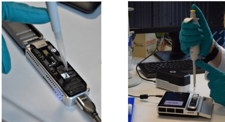
Figure 1.4: Oxford Nanopore MinION portable Sequencing Devices: Left: MinION MK1B [30]; Right: MinION MK1C. Compared to MK1B, MK1C contains an embedded GPU for basecalling on device [31].
