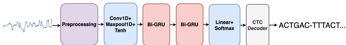
Figure 2.5: Overview of the DeepNano-Blitz architecture. The architecture consists of preprocessing, convolutional, and bidirectional LSTM/GRU blocks, followed by a linear output layer and CTC decoding.
