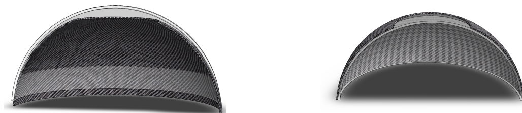
(a) A negative mold where the carbon fiber plies are placed inside the dome.
