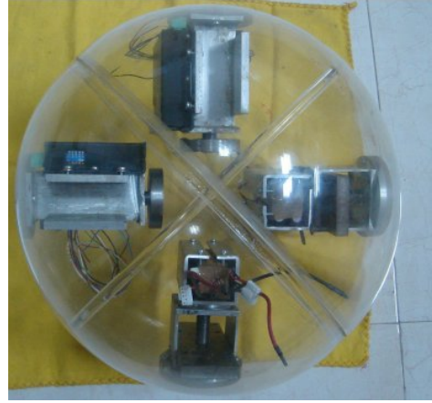
(b) V. Joshi's spherical robot with two motors. Image reprinted from [17].
