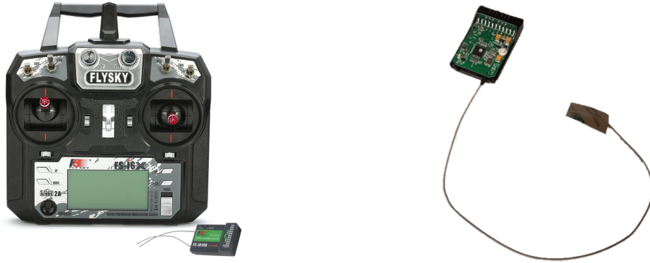
(a) Flysky FS-i6X 2.4GHz remote control and receiver. Image reprinted from Amazon. (b) RC receiver modded to connect an antenna further away from the body.
