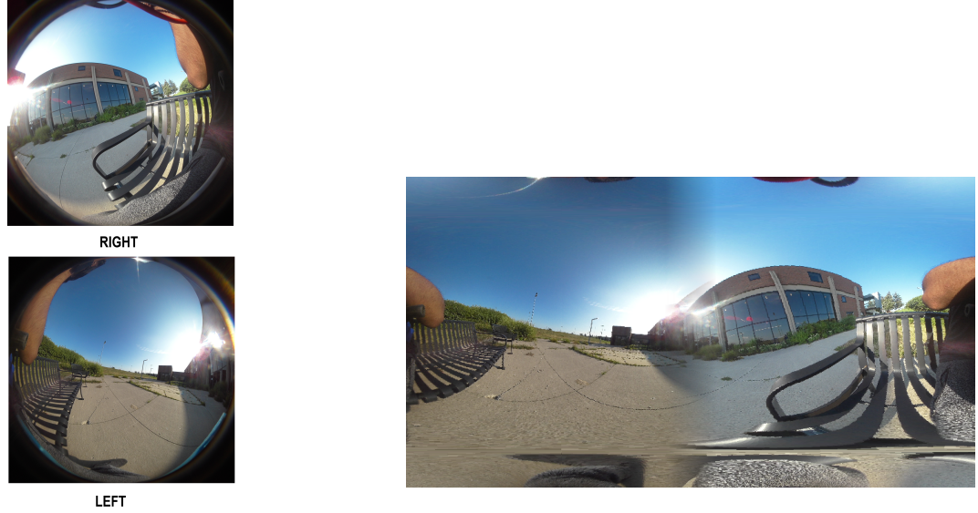
(a) Raw image captured from left and right Kodak cameras. (b) Image after dewarping and blending.
