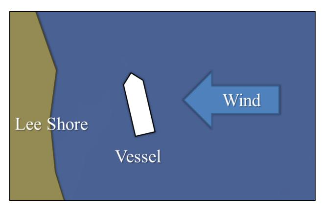
**Fig. I.6.** Location of a lee shore or coast. In sufficiently high winds, the vessel depicted would be in peril. The "lee side" of this ship is to the left, while the "weather side" is on the right. The Dictionary of English Nautical Language, accessed 28 February, 2014, <u>http://www.seatalk.info/cgi-bin/nautical-marine-sailing-dictionary/db.cgi?db=db&uid=default&FirstLetter=l&sb=Term&view\_records=View+Records&nh=3</u>
