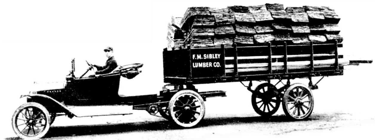
(c) August Fruehauf's 1914 Semi-Trailer on a Modified Ford Model T (Strohl, 2017)
