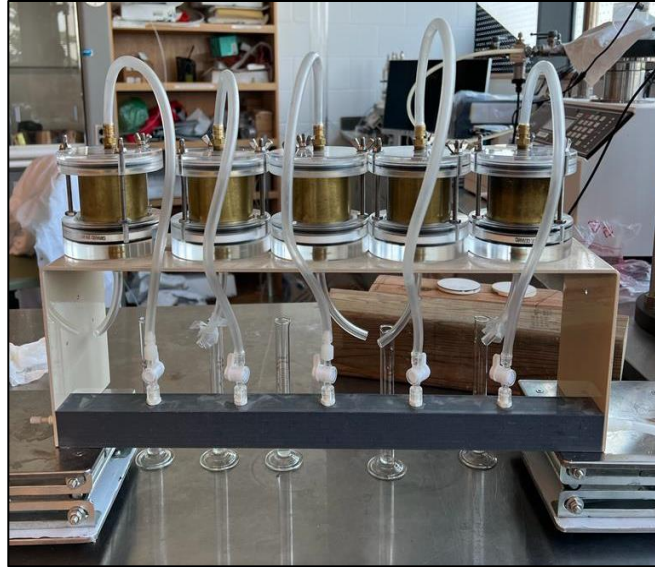
Figure 4.2: Tempe Cell experimental set up
