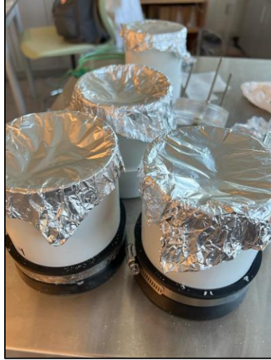
Figure 4.1: Columns used for ECw experiments
