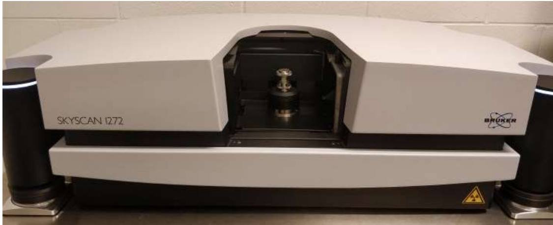
Figure 23 The Bruker Skyscan 1272 (CMOS Edition) micro-CT system, a high-resolution x-ray microscope [114].
