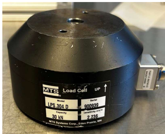
Figure 15 The 30 kN Load Cell used during tensile and compressive testing.
