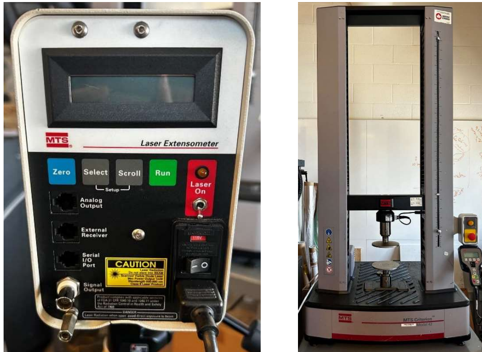
Figure 14 From left to right: LX 500 High Resolution Laser Extensometer [112]; MTS Criterion™ High Peak Force Universal Mechanical Tester [113], in compression mode.
