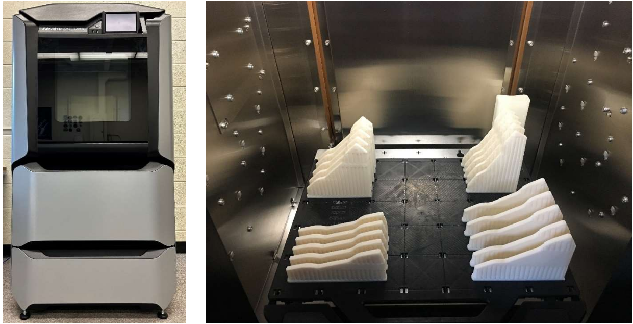
Figure 7 Stratasy F370 FDM 3D printer and tensile specimens encased in SR-30 [111] support structure.
