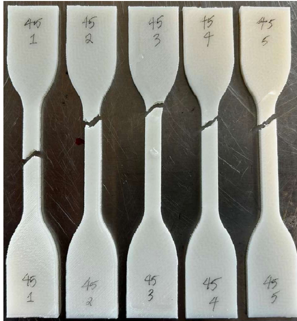
Figure 18 Five tensile specimens with 45° print orientation after fracture.
