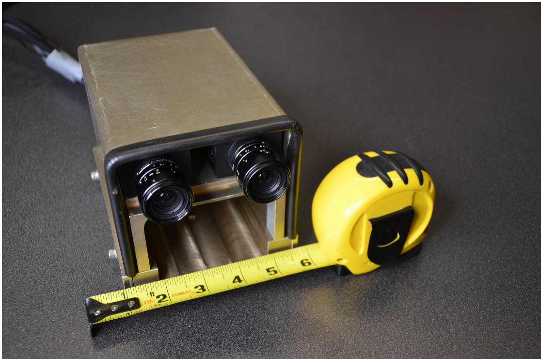
Figure 4.1: Stereo Sensor. Two calibrated video cameras are mounted in a metal enclosure. See text for details.
