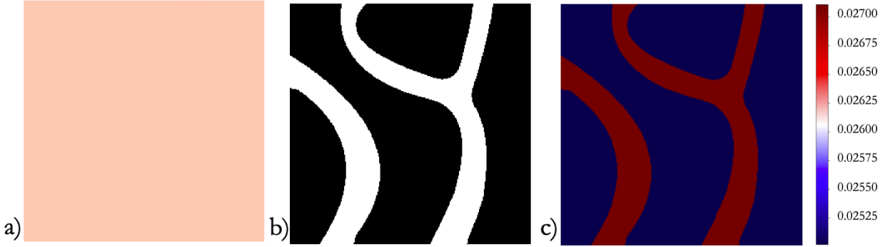
Figure 6.12: Simulated skin tissue with two embedded curved vessels at different depths with the same hemoglobin volume fraction and recovered hemoglobin distribution using inverse chromophore map f_{GP} . a) The simulated skin generated from \theta_m = 0.04 , \theta_h = 0.025 with two embedded curved vessels at depth d = 0.2 cm, and d = 0.25 cm, respectively, with vessel \theta_h = 0.0275 in each. b) The embedded vessel schematic. c) Recovered hemoglobin distribution and distinguished blood vessels.
