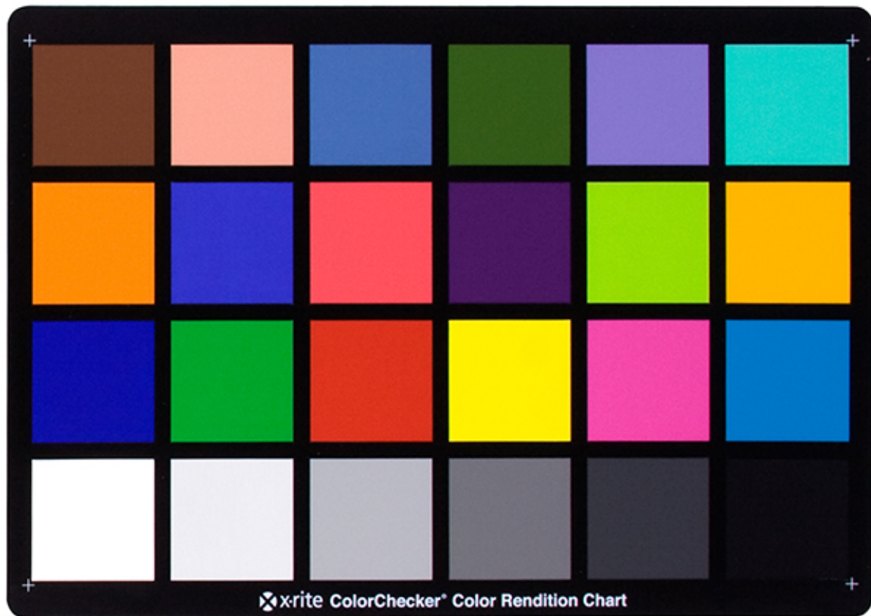
Figure 5.3: Macbeth 24 swatch ColorChecker chart. Each colour swatch is manufactured to have precise known spectral reflectance for colour constancy and accuracy in digital photography.
