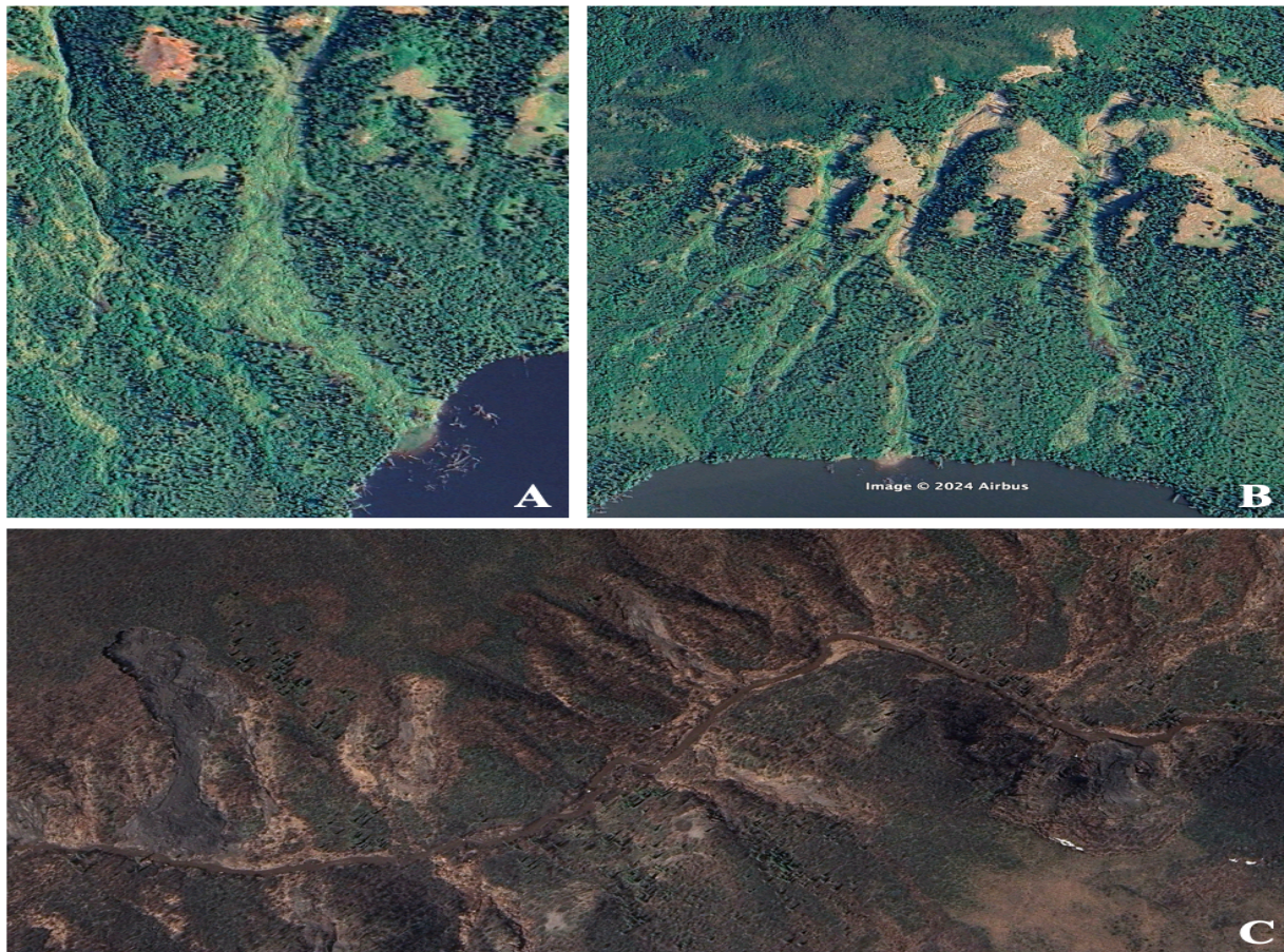
Figure 9: Primary landsliding features affecting the impacted lakes. Caribou 2 - single active layer detachment slide (a), Caribou 3 - active layer detachment slides at the northern end of (b) Douglas - retrogressive landslides up creek (c)
