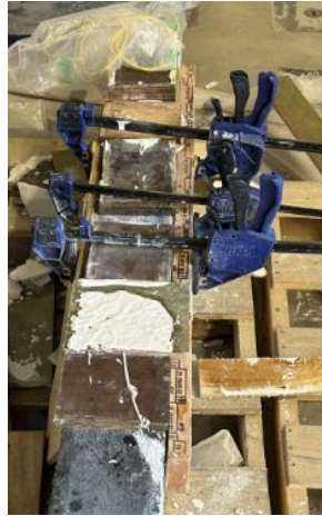
Figure 4-6. Plaster Placement on Loading Points
