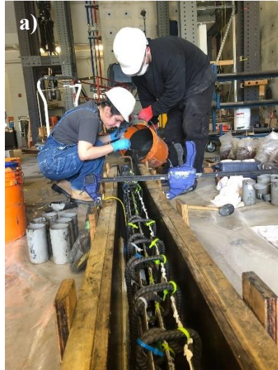
Figure 3-17. Pouring of UHP-FRC into Beam Specimen Formwork
