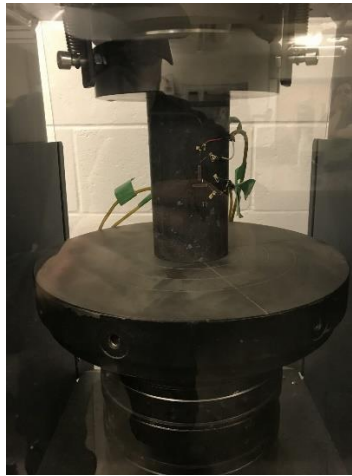
Figure 3-22. Cylinder Instrumented with Strain Gauges in Compression Tester
