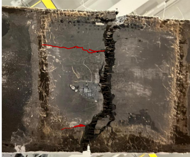
Figure 4-17. Bond Splitting in Bottom Cover of B1R2.3-1
