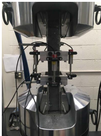
Figure 2-6. Direct Tension Test Setup (From Voss et al., 2022)
