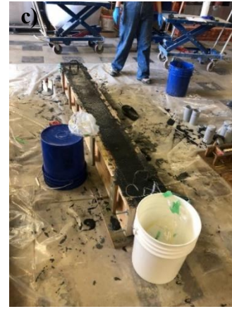
Figure 3-16. Finished Pour of UHP-FRC in Formwork
