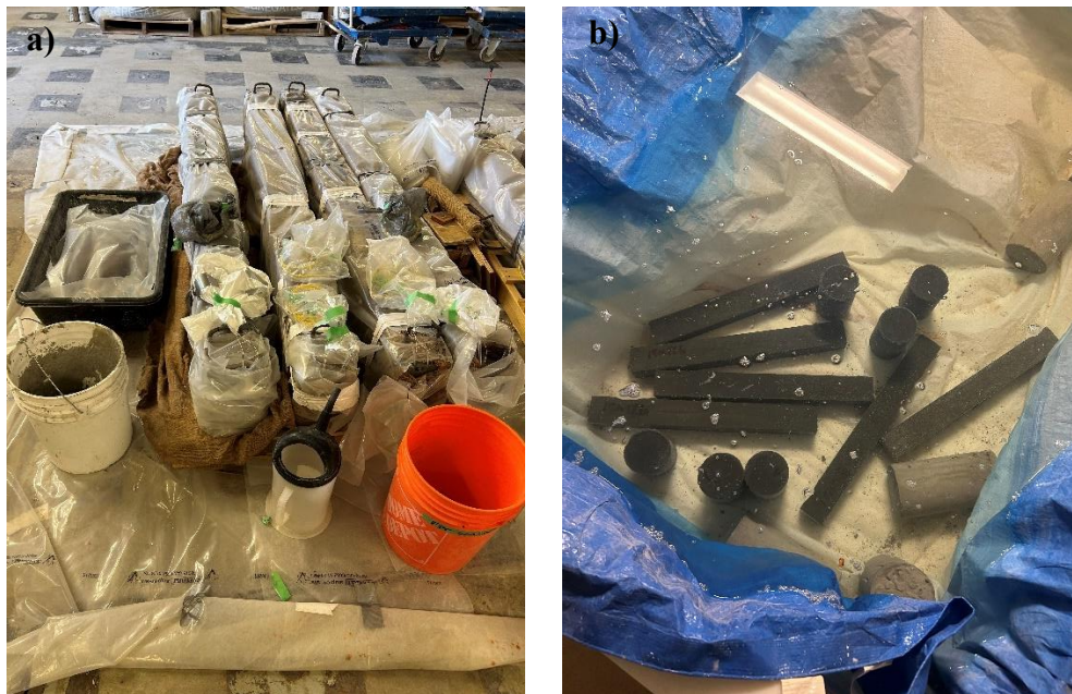
Figure 3-20. a) Curing of Beam and Companion Specimens and b) Curing of 28-Day Test Material Characterization Specimens
