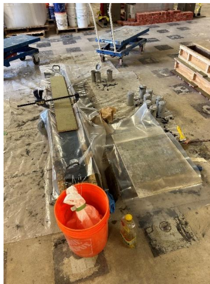
Figure 3-19. Finished Casting of a beam specimen and accompanying material characterization samples
