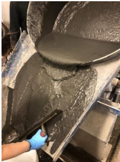
Figure 3-13. Removal of UHP-FRC from Mixer
