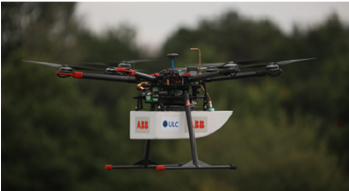
Figure 1.9: The ABB Inc. OA-ICOS instrument, which is attached to a hexacopter. This instrument is compact and robust, allowing for easy deployment and operation when taking highly sensitive measurements of methane. The instrument will be developed for the Martian climate and will be able to reliably detect sub-ppbv measurements of methane on Mars on an hourly scale.
