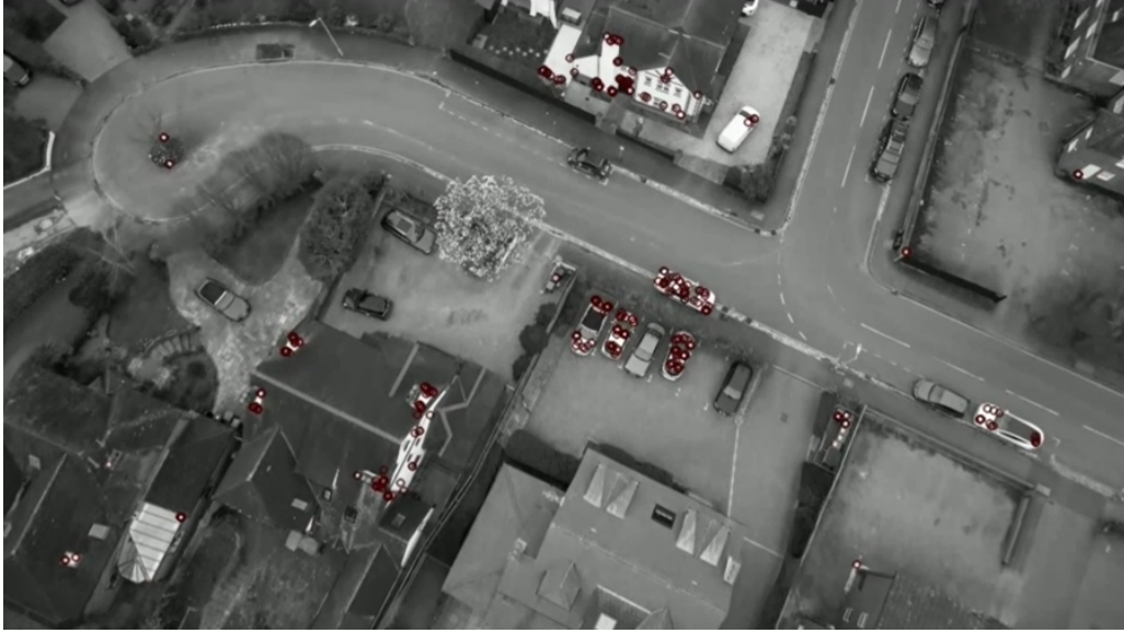
Figure 8: ORB feature candidates detected in a representative frame. Many features are spatially clustered or redundant, motivating learned feature selection.
