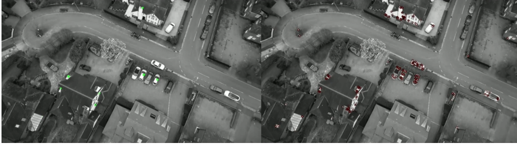
Figure 24: Qualitative comparison of feature detection on a representative frame. Right: classical ORB feature detection showing dense and redundant features. Left: CNN-based feature selection retaining fewer but more stable and well-distributed features.
