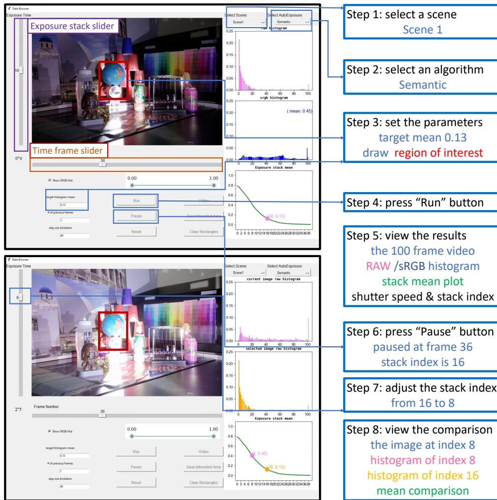
Figure 4.1: The basic steps for using our AE platform. The user selects a scene and an algorithm. The parameters of the AE algorithm can be adjusted. After the AE algorithm runs, the platform plays the output images and the corresponding plots at 10 FPS. The user causes "pause" at any time frame to adjust the exposure stack slider for comparison. Image histograms for each frame are also shown.
