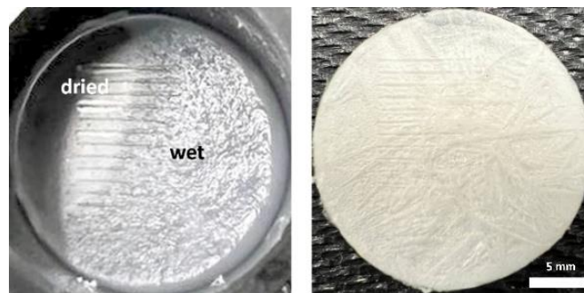
Figure 3-17: Porous and nonporous zones through controlled drying on a sample with a part heated more on a hot plate.
