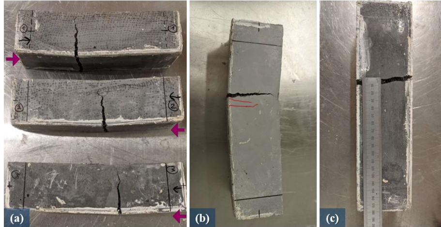
Figure 5.16: (a) Fractured specimens (b) multi-cracking in the constant moment region for specimen #3 and (c) measured crack width
