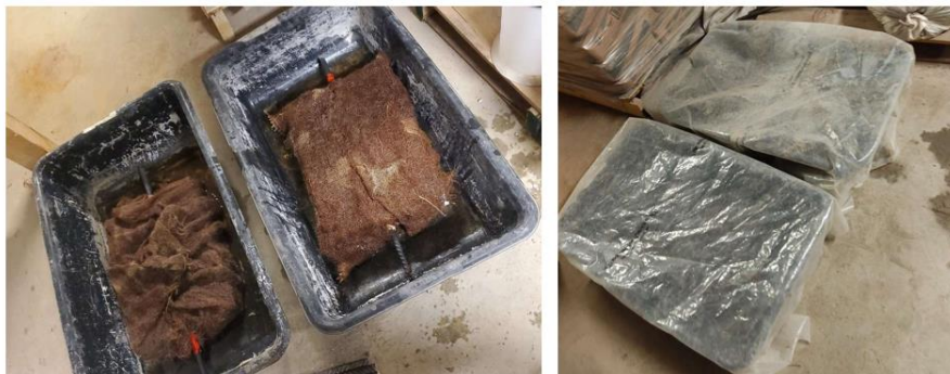
Figure 6.7: Moist curing of DTP specimens for 28 days
