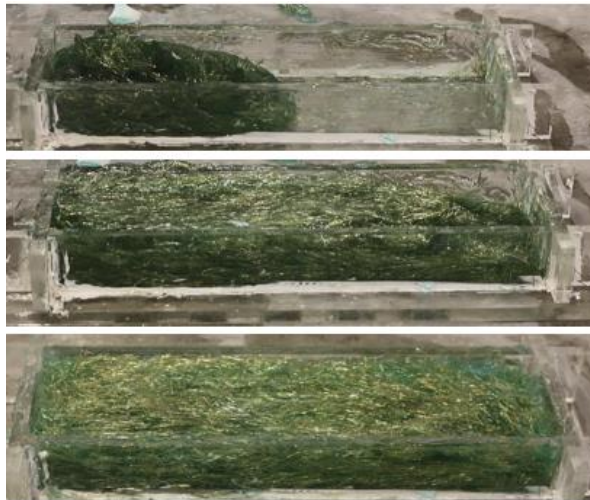
Figure 4.44: Flow timeline of flow from one end for 0.3CM2 in FR formwork
