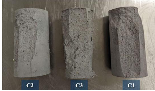
Figure 5.5: Fracture pattern of failed unreinforced cylindrical specimens
