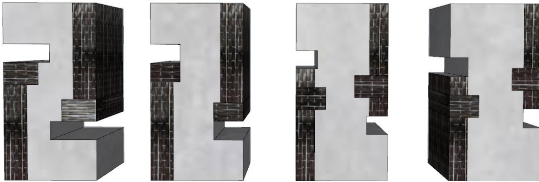
Figure 7.5: Push-off specimens wrapped with CFRPs
