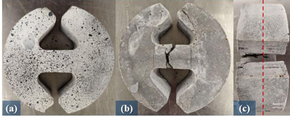
Figure 9.46: Fractured specimen due to out of plane bending (a) front view, (b) back view and (c) side view
