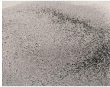
Figure 3.3: Unburnt coal grain residues in FA-F
