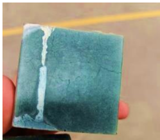
Figure 3.11: Drying Shrinkage cracking patterns on a discolored GGBFS-based mortar
