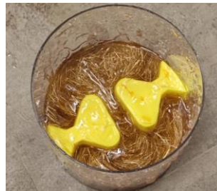
Figure 4.42: Formation of weak plane in MS specimens cast with flow from one end
