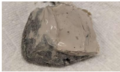
Figure 3.10: MK-750 based geopolymer matrix specimen demonstrating setting and segregation issues
