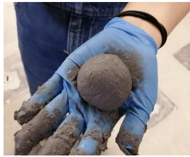
Figure 3.23: Highly thixotropic concrete through use of RCA in GPC3 mixes
