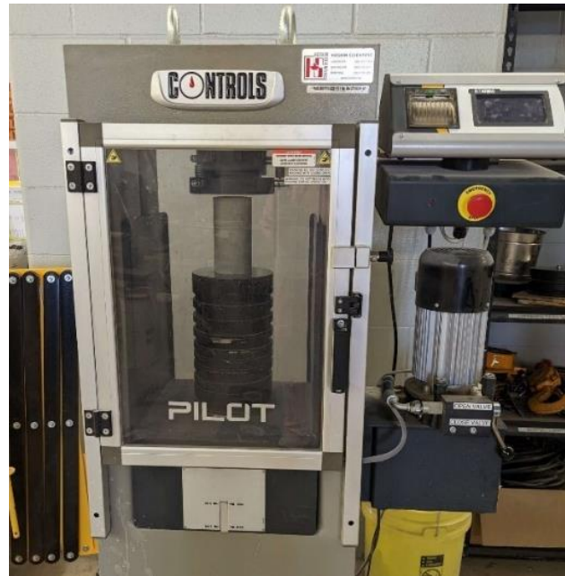
Figure 5.4: Controls Compression Machine used for uniaxial compression of unreinforced geopolymer concrete cylinders and cubes
