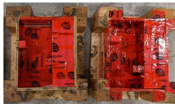
Figure 7.3: Formworks for specimens CS63 and CS34
