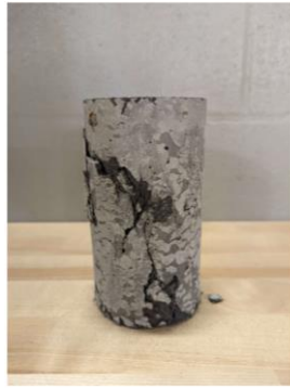
Figure 10.3: Fracture Pattern of nanoengineered UHPFRC in compression
