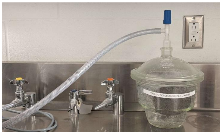
Figure 5.39: Specimens curing in desiccator filled with distilled water and vacuum.
