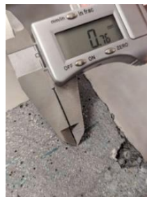
Figure 4.11: Deformation of fiber trace due to saw blade
