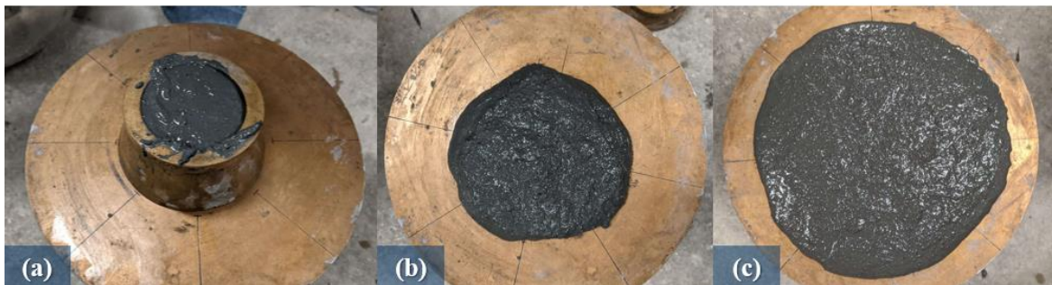
Figure 5.3: (a) Filling the mold with one layer of fresh geopolymer, (b) static spread after 2 minutes, and (c) dynamic spread after tapping
