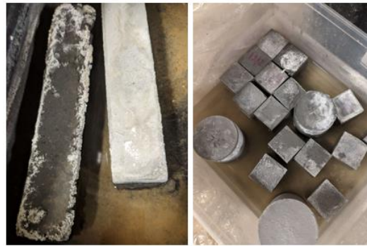
Figure A.9: Efflorescence observed on early mixes with SSSH1.5
