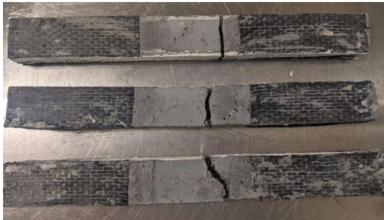
Figure 5.21: Failure planes of THFRGC direct-tension specimens
