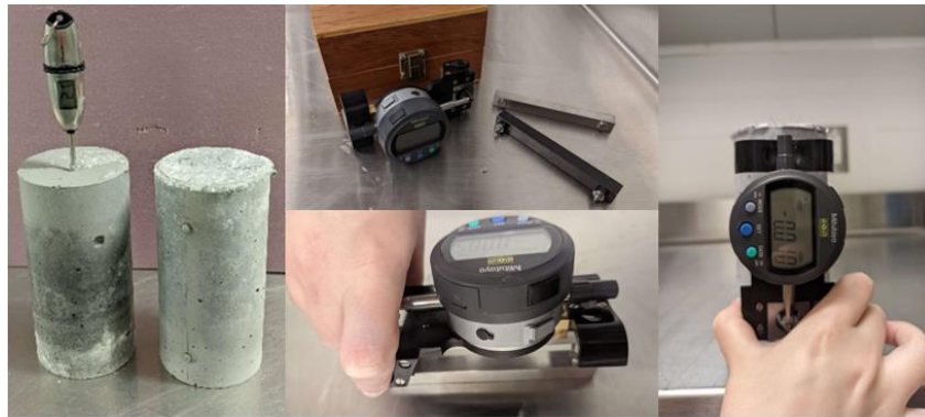
Figure 5.34: Preparation of specimens for CTE test and measurement of length change with DEMEC gauge
