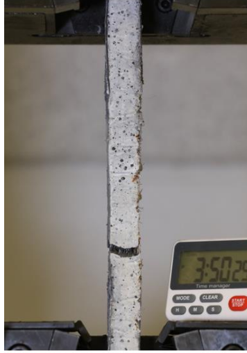
Figure 10.4: Failure of nanoengineered UHPFRC in tension
