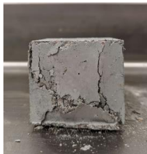
Figure 5.11: Fractured THFRGC cube after uniaxial compression test
