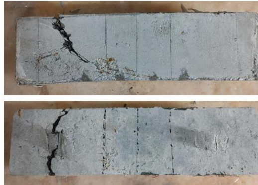
Figure 10.21: Shear failure between an input and output electrode for specimen FP2-B
