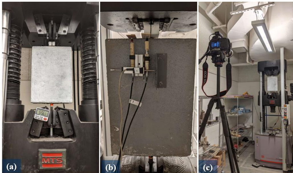
Figure 6.12: (a) MTS Criterion test frame, (b) Back face of specimen with attached hardware components (c) Camera and lightning setup for DIC analysis
