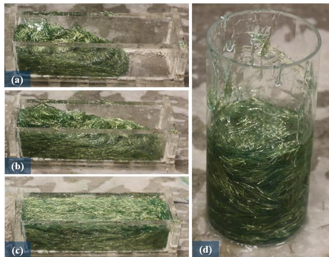
Figure 4.46: One way casting of 0.3CM2 (a-c) Flow timeline in CS formwork, (d) fiber distribution in C1
