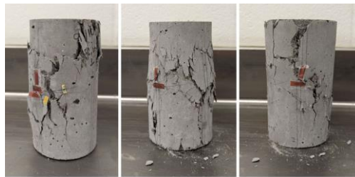
Figure 5.9: Fracture mode of cylindrical geopolymers THFRG specimens
