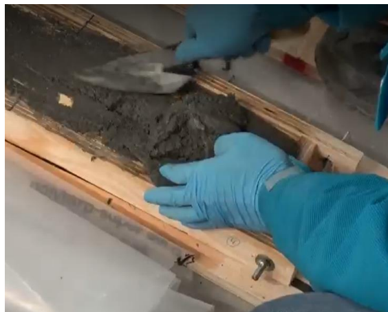
Figure 4.22: Surface finishing by scrapping excess UHPFRC for LD1 mix
