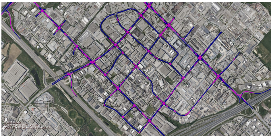
Figure 8- VISSIM Link-Connector Structure
